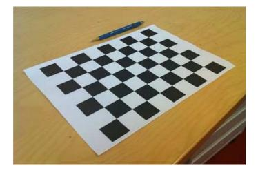
Figure 6: Calibration pattern
