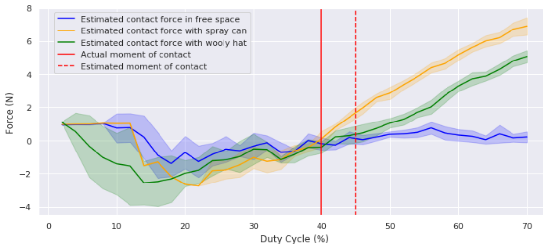
Figure 5.15 The figure shows the estimated contact force when the finger bends in free space (blue line) and when the finger makes contact with the spray can (orange line) and the woolly hat (green line). The red line shows the moment when the contact actually happens while the red dashed line shows the moment when the system detects the contact.
