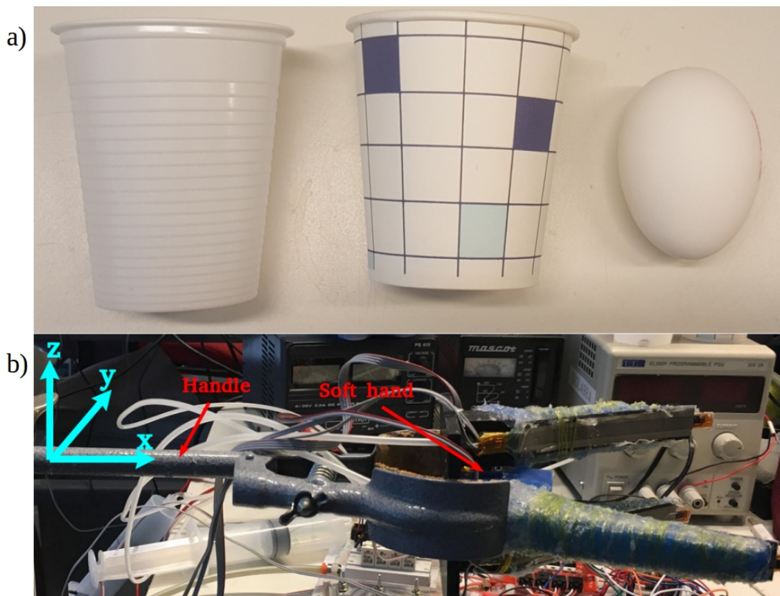
Figure 5.21 (a) The target objects in this experiment: an empty plastic cup, an empty paper cup, an empty eggshell (left to right). (b) The soft hand setup for this experiment.
