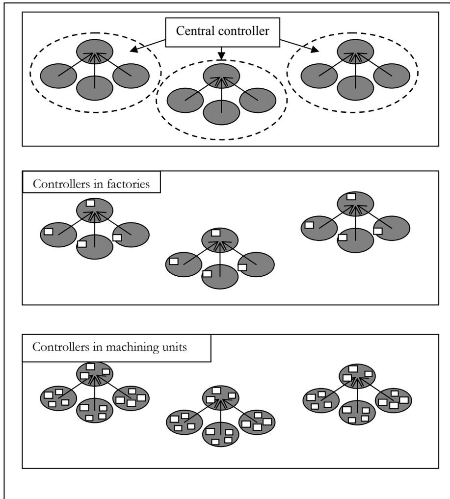
Figure 5-4 Preprogrammed options of centralized, decentralized and distributed control in production networks
