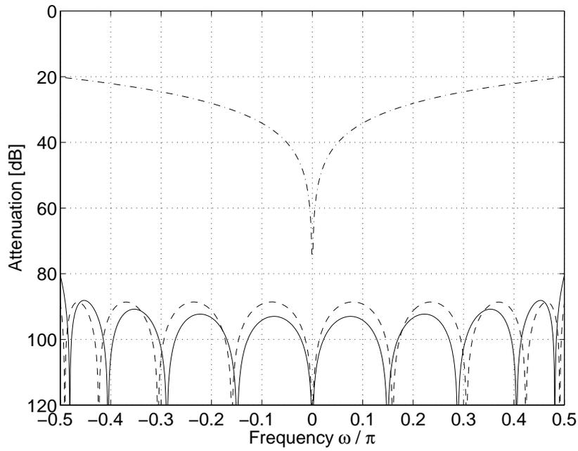
**Figure 6–3:** Image signal attenuations of the IC based enhanced second-order sampling scheme for LS (solid) and minimax (dashed) optimized compensation filters for  $N = 4$  and  $f_s = 50$  MHz. Also shown is the image attenuation of the basic second-order sampling technique (dash-dotted).
