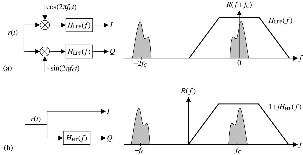
**Figure 2-2:** Extraction of the positive frequency component of a bandpass signal  $r(t)$  using (a) complex exponential oscillator signal and two lowpass filters, (b) the Hilbert filter (band splitter) approach. In both cases, the key element is the  $90^\circ$  phase shift between the  $I$  and  $Q$  branch signals.
