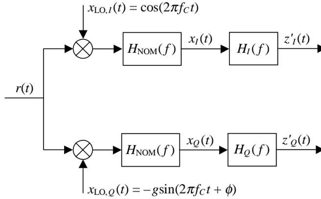
**Figure 3–3:** Imbalance model for the analog front-end processing.
