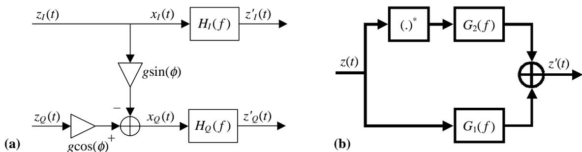
**Figure 3-4:** Wideband signal model for front-end imbalances in terms of (a) real-valued and (b) complex-valued signals.
