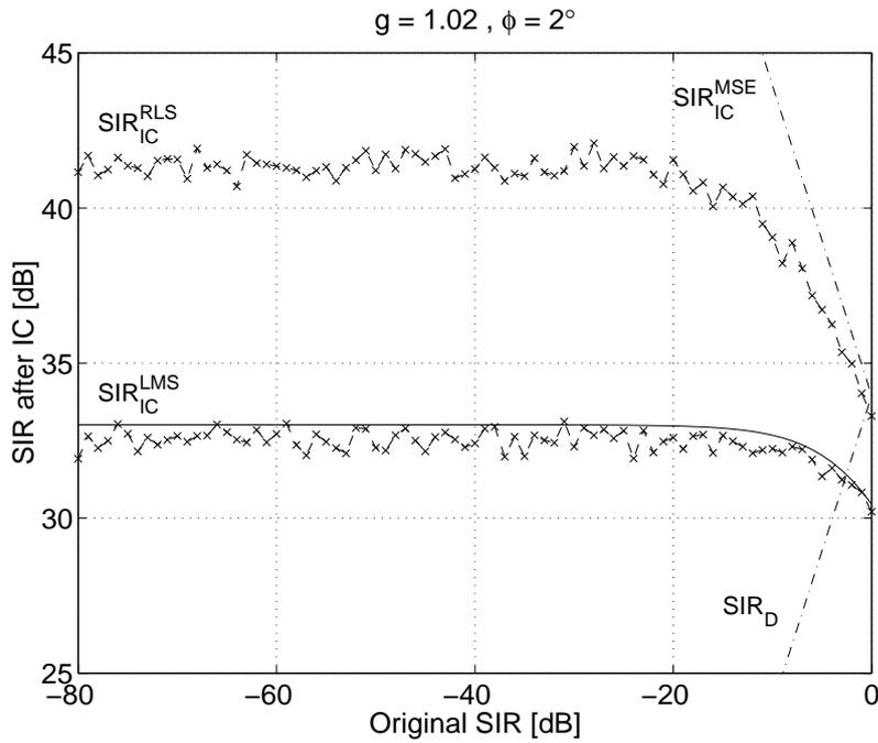
**Figure 4-4:** Theoretical (solid) and simulated (x-marked) interference canceller steady-state SIR performances,  $\mu P_V = 10^{-3}$  (LMS) and  $\lambda = 1.0$  (RLS). Both the desired and image signals are QPSK modulated, timing error of half of the symbol interval and additive noise of SNR = 10 dB included.
