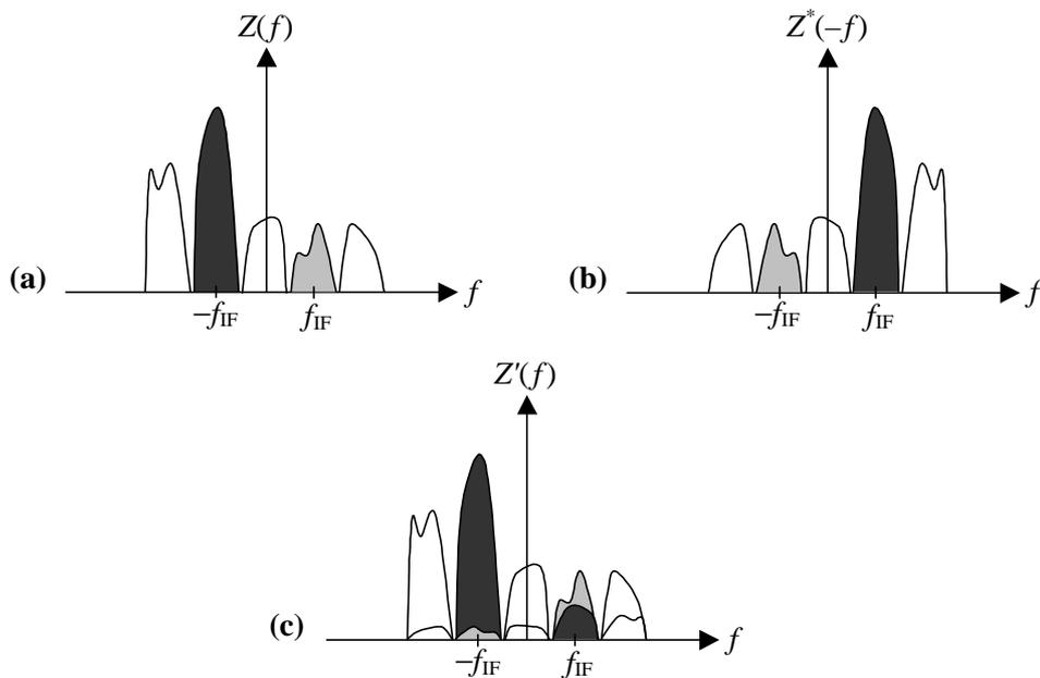
**Figure 3–5:** A frequency domain illustration of the basic imbalance effect.
