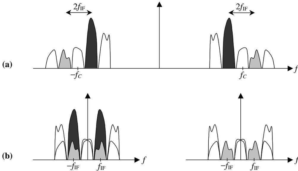
**Figure 3–1:** (a) A frequency domain illustration of the received signal. A specific channel signal (grey) and its image signal (dark) are separated by  $2f_{IF}$  and are illustrated in different colours. (b) The spectrum of the downconverted signal after real mixing and lowpass filtering without (left) and with (right) image rejection filtering.
