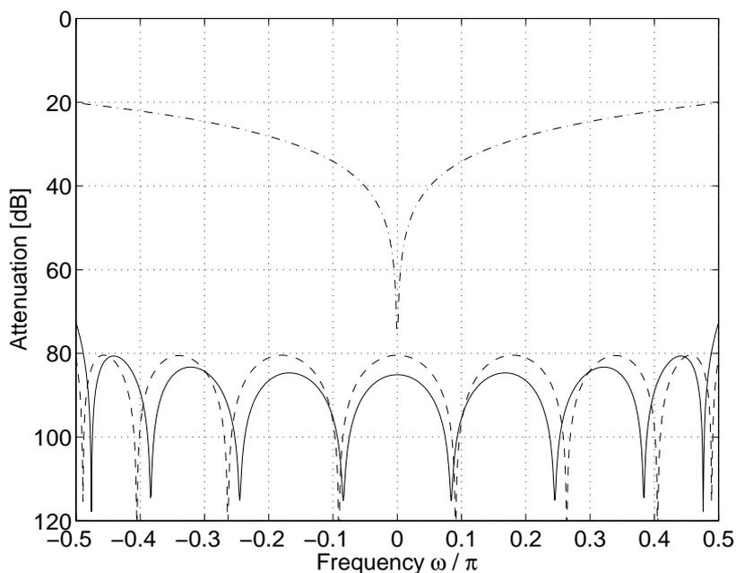
**Figure 6–5:** Image signal attenuations of the FD filter based enhanced second-order sampling scheme for LS (solid) and minimax (dashed) optimized compensation filters for  $N = 4$  and  $f_s = 50$  MHz. Also shown is the image attenuation of the basic second-order sampling technique (dash-dotted).
