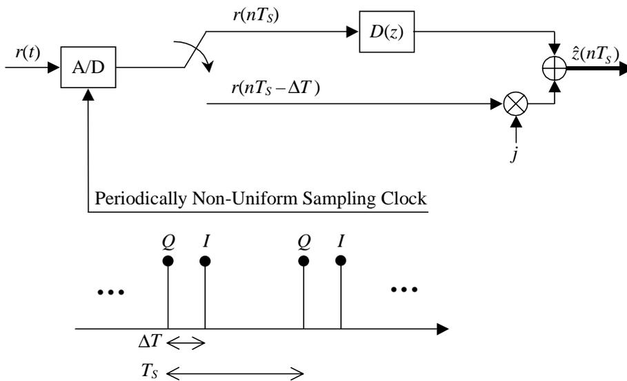
**Figure 6–4:** Enhanced second-order sampling scheme based on fractional delay filtering. Through periodically non-uniform sampling, only one actual A/D converter is needed.
