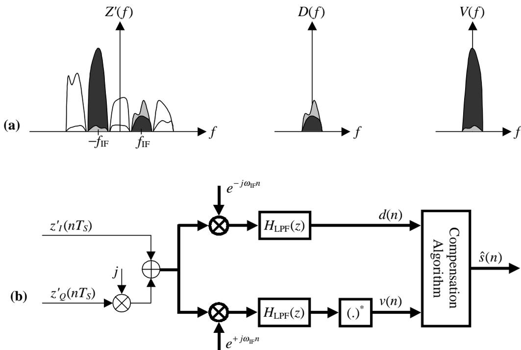
**Figure 4-1:** Baseband observation generation for digital imbalance compensation. (a) The spectra of  $z'(t)$  and the resulting baseband observations  $d(t)$  and  $v(t)$ . (b) The corresponding digital implementation structure where complex-valued processing is depicted in bold.
