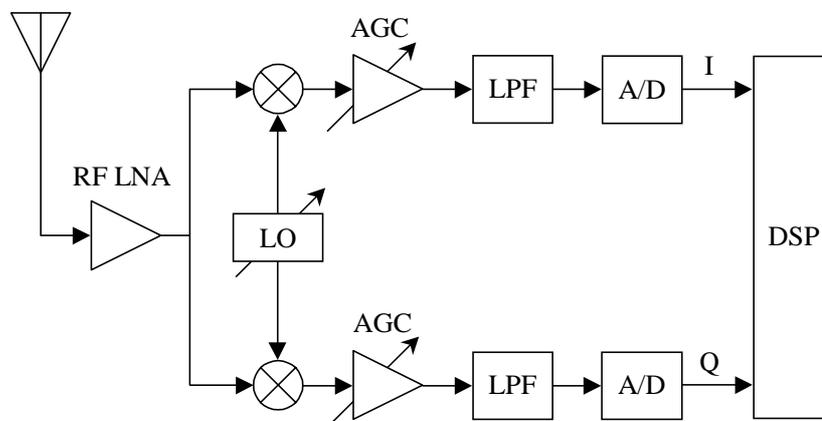
**Figure 1–1:** General I/Q processing based receiver structure.
