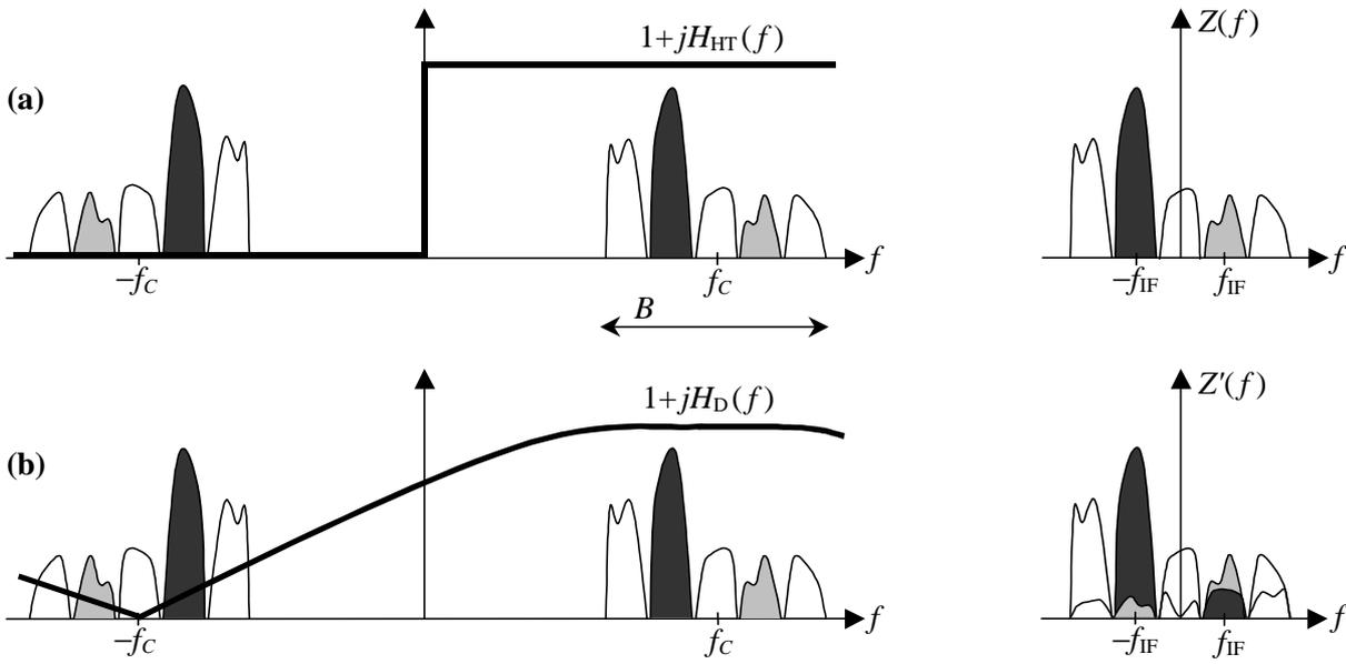
**Figure 6–1:** A frequency domain illustration of the basic relation between the ideal I/Q sampling (a) and its second-order sampling based approximation (b) in case of multichannel downconversion.
