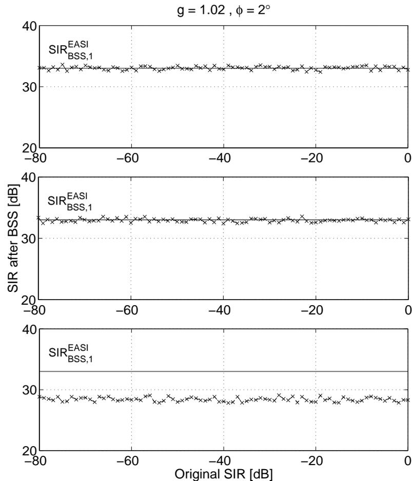
**Figure 4-5:** Theoretical (solid) and simulated (x-marked) signal separator steady-state SIR performances,  $\alpha = 0.002$  (EASI). Both the desired and image signals are QPSK modulated, (a) ideal sampling and no additive noise, (b) ideal sampling and additive noise SNR = 20 dB, and (c) half of the symbol interval timing error and additive noise SNR = 20 dB.
