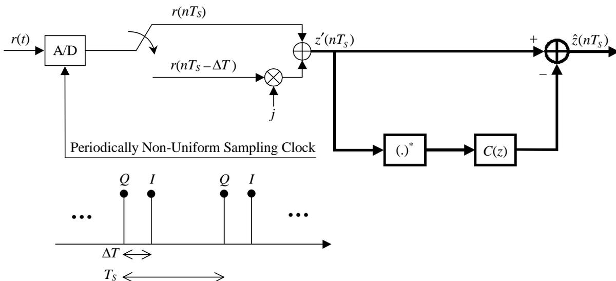
**Figure 6-2:** Enhanced second-order sampling scheme based on fixed interference cancellation. Through periodically non-uniform sampling, only one actual A/D converter is needed.
