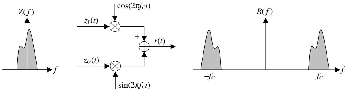
**Figure 2–1:** Bandpass signal transmission.
