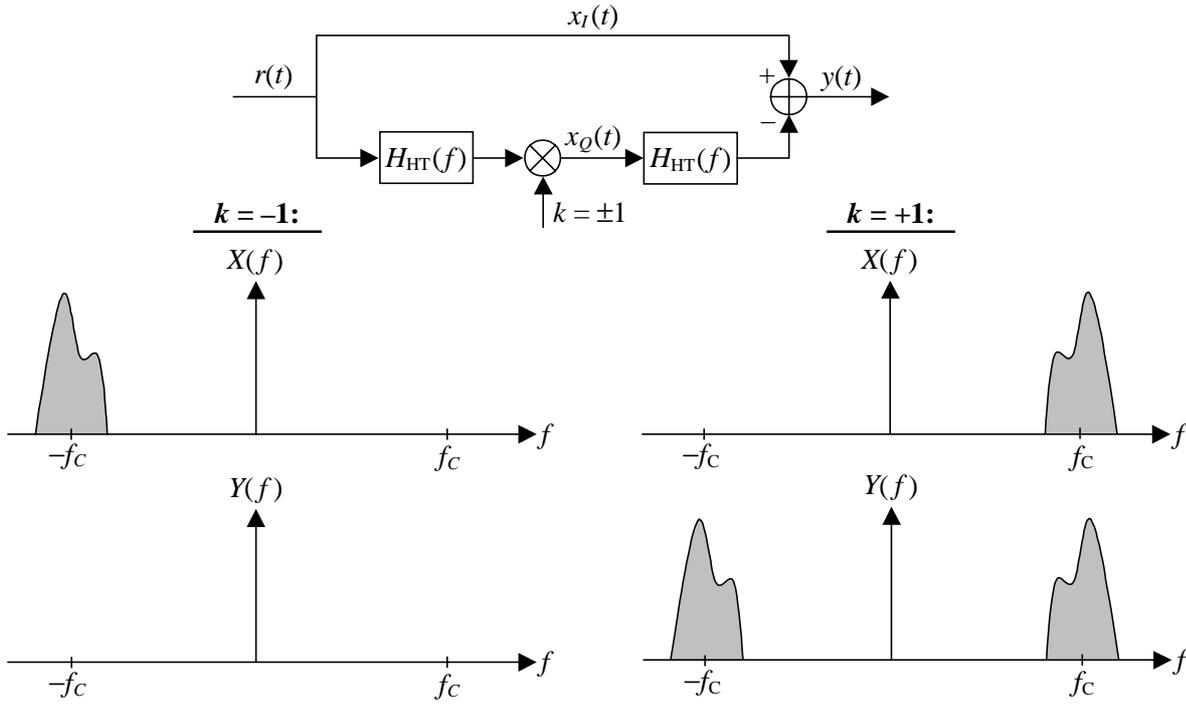
Figure 2–3: Spectral decomposition of a bandpass signal  $r(t)$ .
