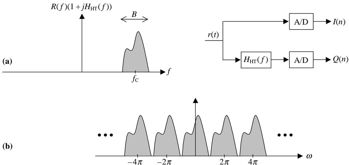
**Figure 5–1:** (a) Formal representation of complex or I/Q sampling. (b) The resulting periodic spectrum of the sampled complex-valued signal  $I(n) + jQ(n)$  for  $f_s = B = f_c/r$ .
