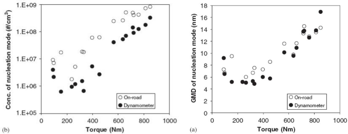
Figure 6.8. Concentration of the nucleation mode particles and GMD of the nucleation mode measured on road and on a chassis dynamometer. The test vehicle was a heavy duty diesel bus equipped with a DOC. Adapted from Paper III.
