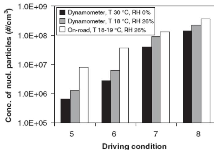
Figure 6.13. Effect of dilution air temperature and RH on the concentration of the exhaust nucleation mode particles. Laboratory measurements on a chassis dynamometer were performed using 12 as the dilution ratio of the primary diluter. The test vehicle was a heavy duty diesel bus equipped with a DOC. Adapted from Paper III.
