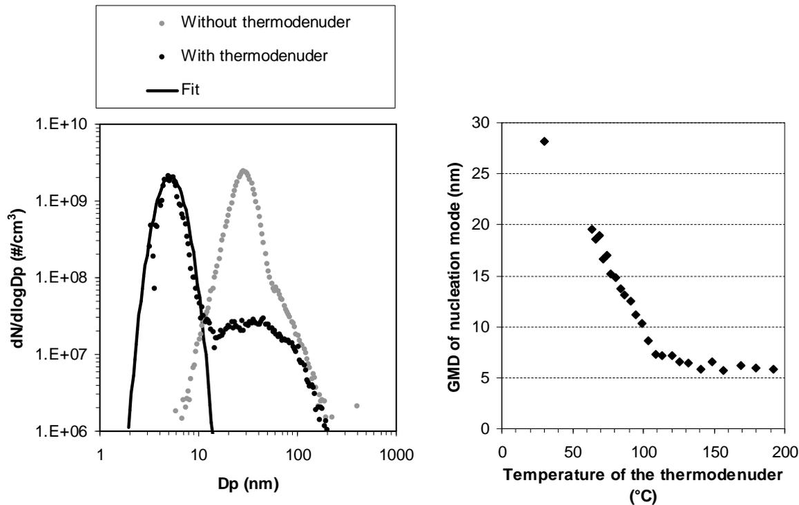
Figure 6.6. a) Particle size distributions in the exhaust plume of the heavy duty diesel truck without exhaust after-treatment. The measurements were conducted on road with and without a thermodenuder at the driving condition 6. b) The nucleation mode GMD as a function of the thermodenuder temperature. Laboratory measurement, driving condition 8. Adapted from Paper IV.
