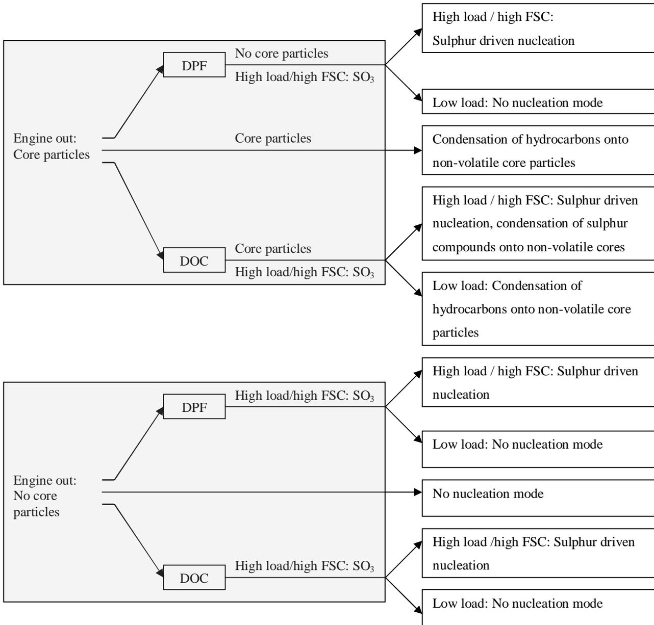
*Figure 7.1. Processes affecting the formation of the nucleation mode when the non-volatile core particles exist (upper) and when the non-volatile core particles do not exist (lower) in raw exhaust.*
