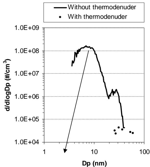
Figure 6.1. Exhaust particle size distributions of a heavy duty diesel engine equipped with a coated DPF with and without the thermodenuder. The arrow shows the change in size distribution when the thermodenuder was switched on (with the thermodenuder, particle concentration was zero, not shown on the log scale). Modified from Paper VI.
