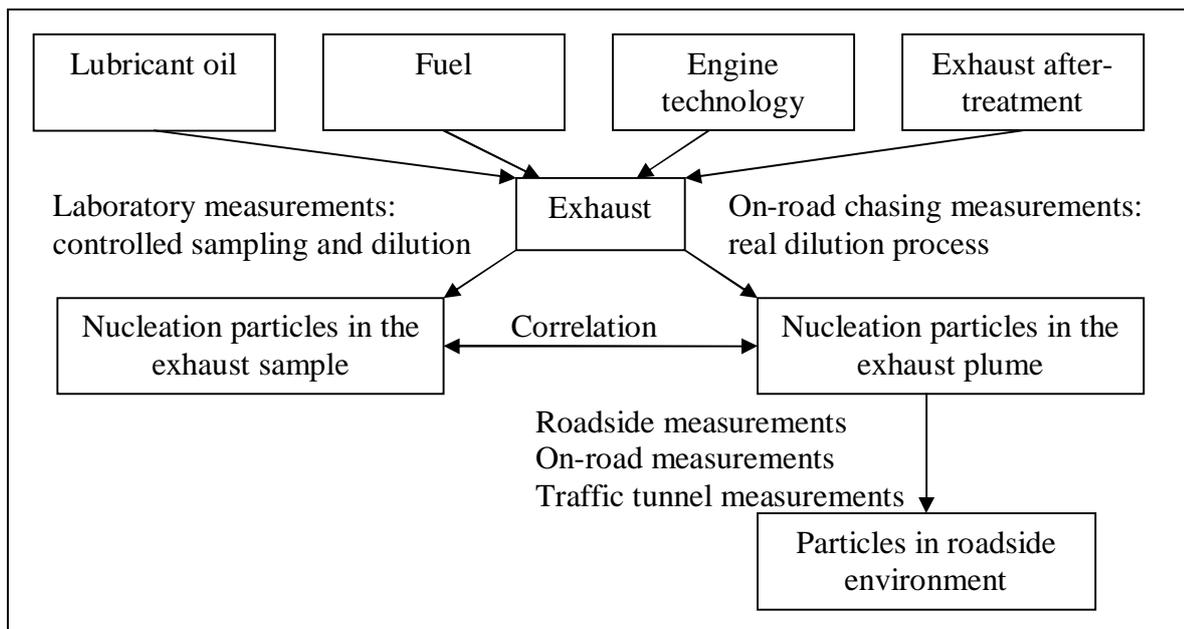
Figure 1.1. Factors affecting the formation of the nucleation mode particles in diesel exhaust and the measuring methods used in the LIPIKA project.
