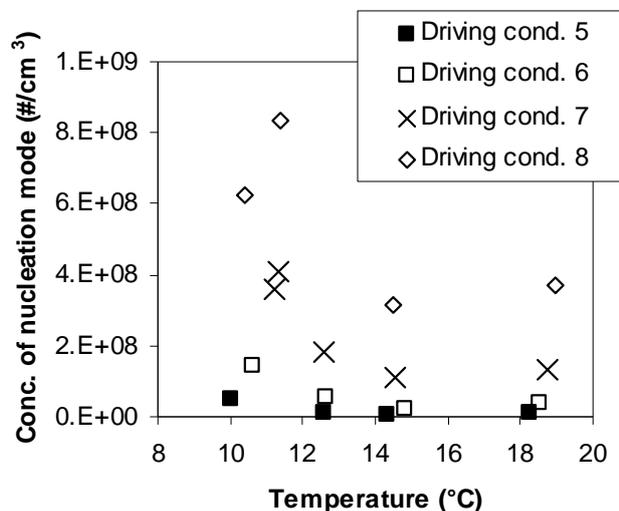
Figure 6.11. Effect of ambient air temperature on the concentration of the nucleation mode particles in the exhaust of a heavy duty diesel bus equipped with a DOC.
