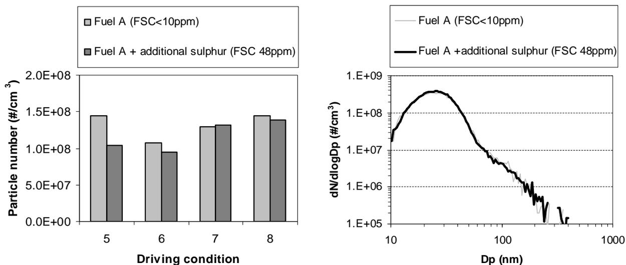
Figure 6.5. a) Exhaust particle number concentration measured with undoped fuel A (FSC<10ppm), and with fuel A doped to FSC 48ppm. The measurements were conducted with heavy duty diesel truck in a vehicle laboratory at four driving conditions of Paper IV. b) Particle size distributions with different fuels (the driving condition 8 of Paper IV).
