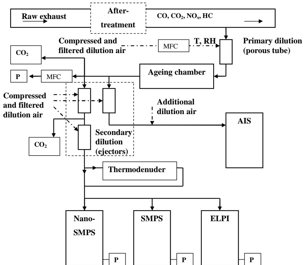
Figure 4.2. The measurement setup used in the laboratory measurements of the diesel vehicles and the diesel engine.
