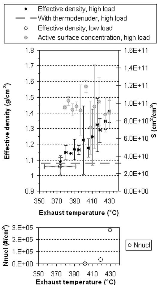
Figure 6.12. The effective density of the accumulation mode particles, the total active surface concentration (upper figure) and the nucleation mode particle concentration (lower figure). A passenger car equipped with a DOC was used at the driving conditions 2 (low load) and 4 (high load) of Paper V. The dashed line shows the effective density of the accumulation mode particles after the treatment with the thermodenuder at the driving condition 4. The measurements were conducted on road.
