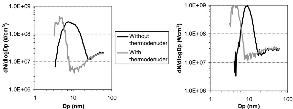
Figure 6.10. Exhaust particle size distributions with and without a thermodenuder for a DOC equipped heavy duty diesel vehicle at the driving condition 7 of Paper III (left side) and for the engine at 75% load (ESC 12) (right side, modified from Paper VI). Laboratory measurements with a Nano-SMPS.
