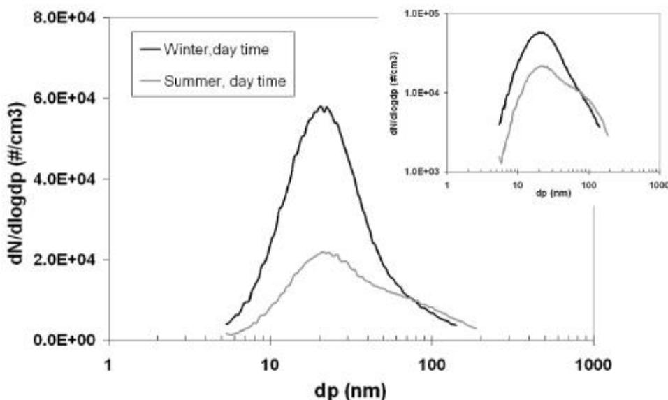
Figure 5.2. Typical particle size distributions measured during rush hours in winter and in summer. In the upper corner the distributions are presented on a log-log scale. Adapted from Paper I.
