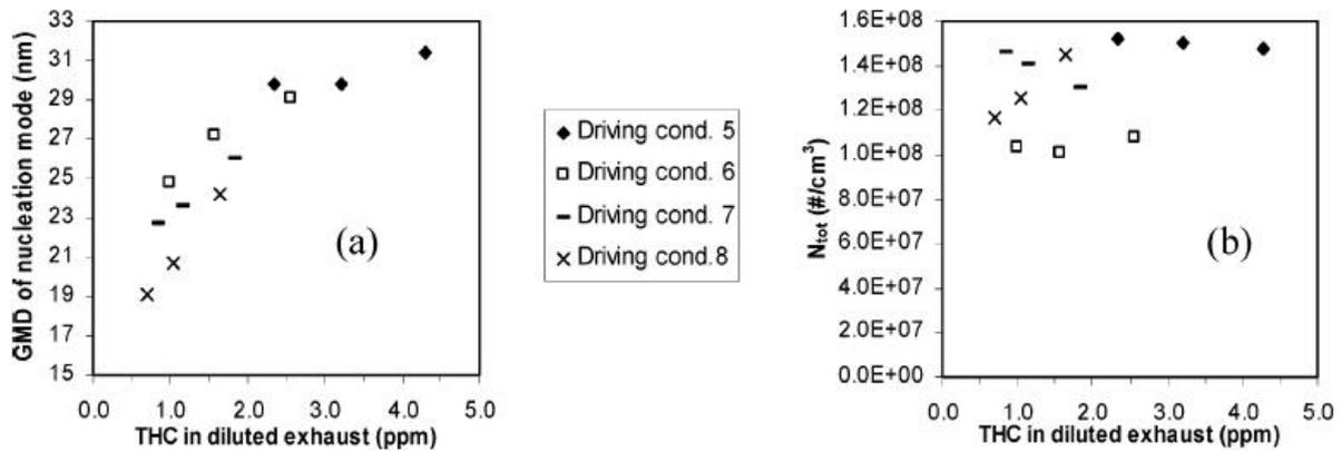
Figure 6.7. GMD of the nucleation mode (a) and the total particle number of exhaust particles in respect of the THC in a diluted sample (in an ageing chamber). Laboratory measurement with a heavy duty diesel truck without exhaust after-treatment. Adapted from Paper IV.
