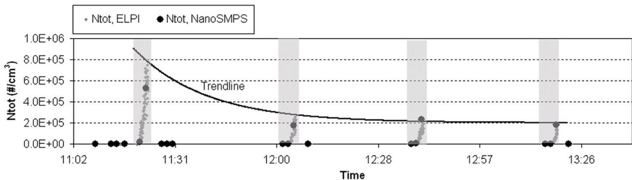
Figure 6.2. Number concentration of the nucleation mode particles in the exhaust plume 8 m behind the DPF equipped passenger car. Measurements were conducted on road at the driving conditions 5 (high load, shaded) and 2 (low load). The test cycle was preceded by long-time driving at low load. Adapted from Paper V.
