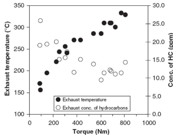
Figure 6.9. Exhaust temperature and exhaust hydrocarbon concentration for an Euro III heavy duty diesel bus. Adapted from Paper III.
