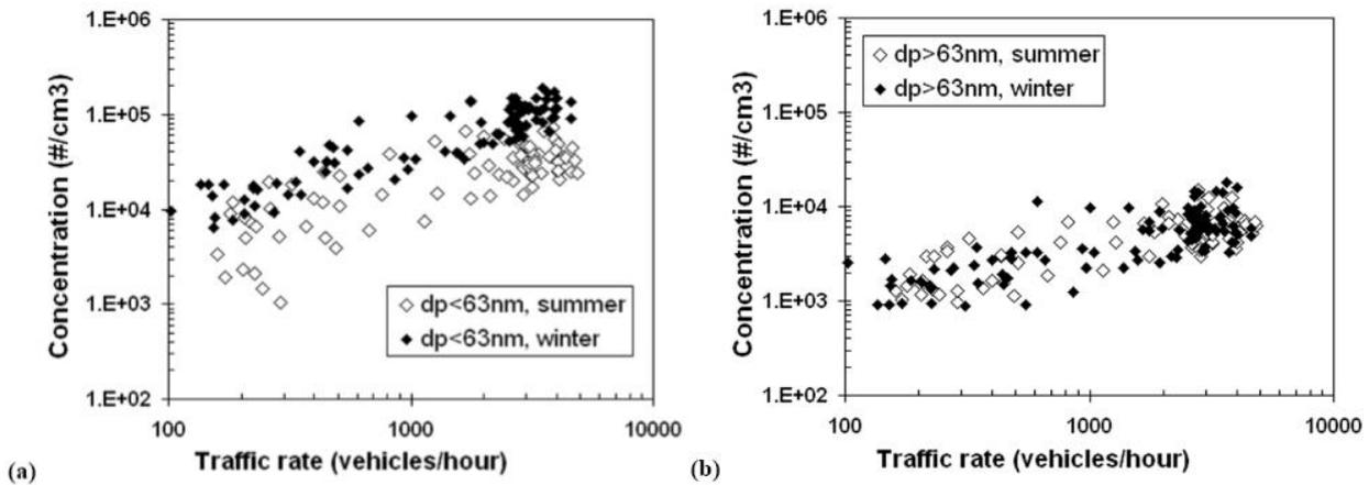
Figure 5.1. Concentrations of two different size fractions as a function of traffic rate: (a) particles smaller than 63 nm, (b) particles larger than 63 nm. Concentrations were measured at a 9 m distance from highway. Adapted from Paper I.
