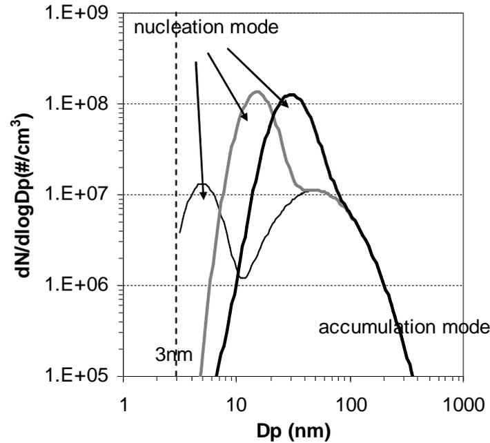
Figure 3.1. Typical particle size distributions of diesel engine exhaust. Three examples for nucleation mode is shown: particle size near the detection limit, nucleation mode and accumulation mode are clearly separable (left pattern); the whole nucleation mode in measurement range, nucleation mode and accumulation mode are clearly separable; nucleation mode and accumulation in nearly equal particle sizes (right pattern). Also typical detection limit (3 nm) is shown.
