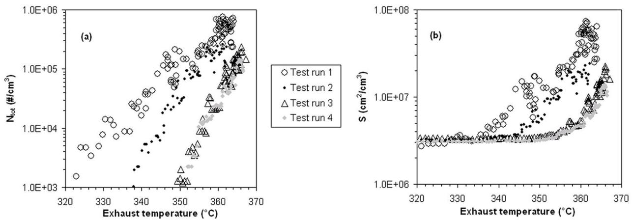
Figure 6.3. Total number concentration (a) and total active surface concentration (b) of exhaust particles in an exhaust plume of the DPF equipped passenger car at driving condition 5. Measurements were made with ELPI in on-road conditions. The exhaust gas temperature measurement was located upstream of the DPF. Adapted from Paper V.
