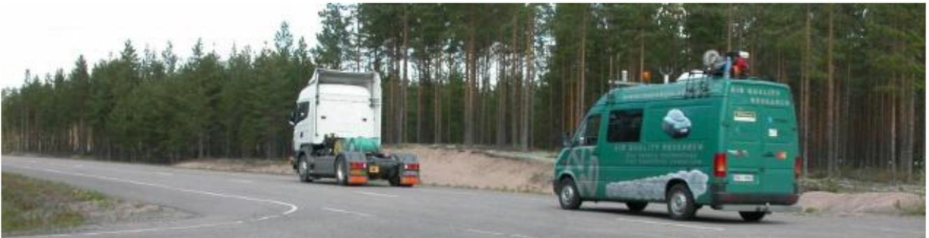
*Figure 4.3. On-road chasing measurement of vehicle particle emission.*
