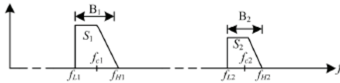
Fig. 4.5 Frequency spectrum of two complex RF signal bands
