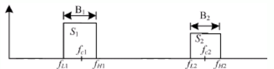
Fig. 4 Frequency spectrum of two complex RF signal bands
