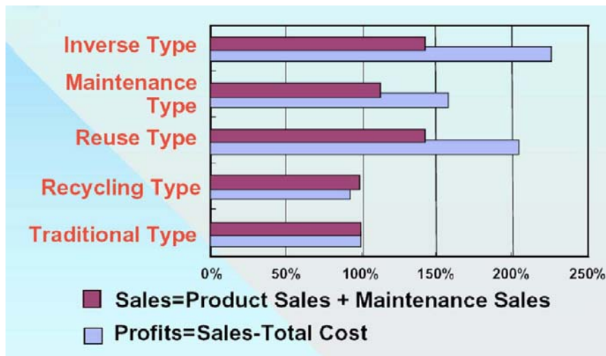
FIGURE 133. The creation of sales and profit in the various life-cycle types. [Umeda, Nonomura & Tomiyama 2000]
