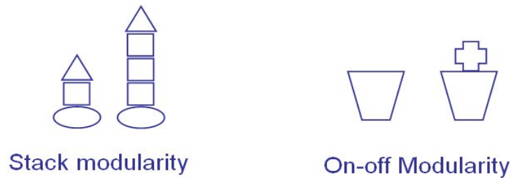
FIGURE 38. The suggested additional types of modularity. Thomas Miller and Per Elgård introduce stack modularity in their research [Elgård & Miller 1998 and Miller & Elgård 1999]. The idea of on-off modularity emerged at a meeting of PhD students at the Danish University of Technology (DTU) in 1998.
