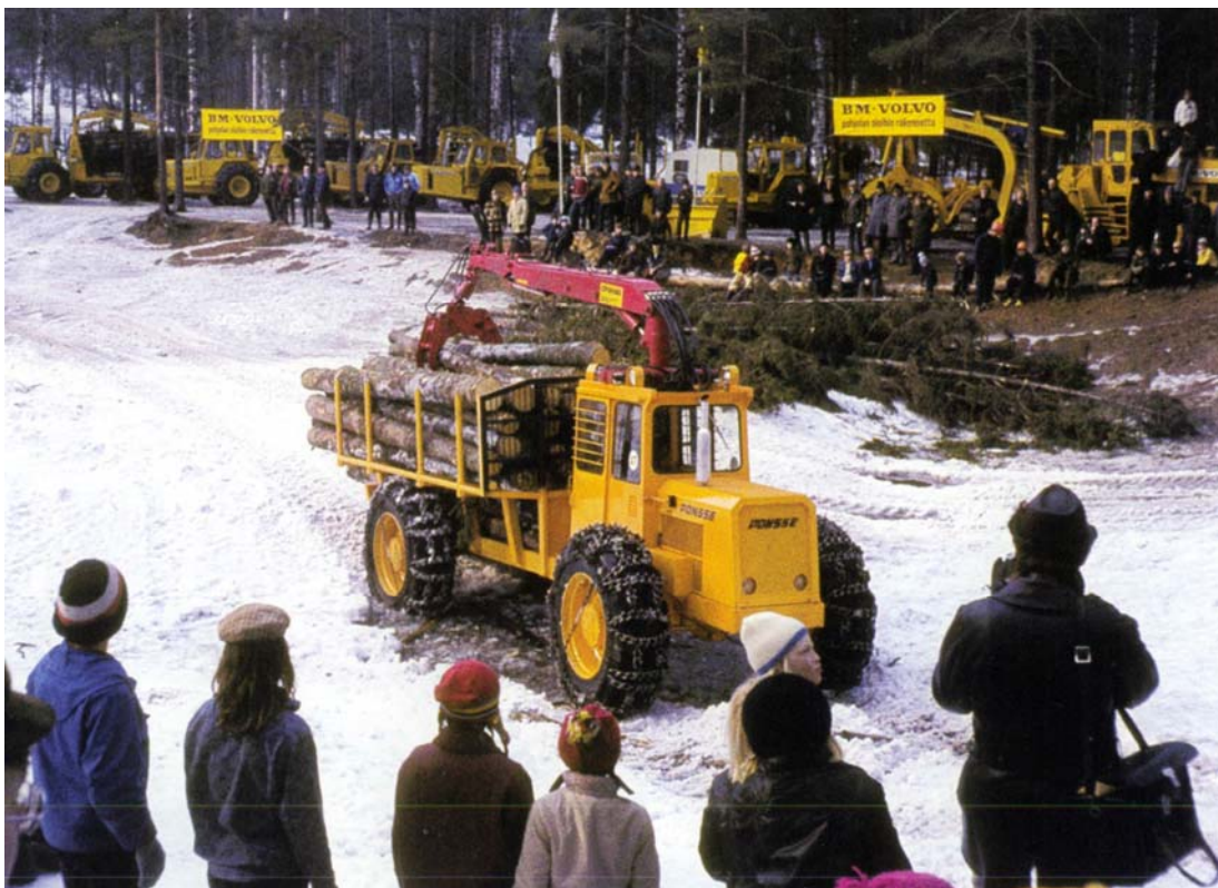
FIGURE 126. The figure shows the first-generation "Ponsse" at a forestry machine fair in the early 1970s. This product was not systematically configurable. The machine structure was improved and developed from one delivery to another. Desired changes or new properties could also be added for each customer. [Kellberg 2000 p 55]
