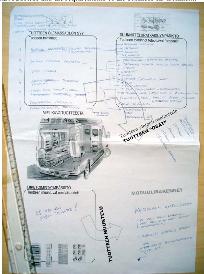
FIGURE 122. A work book with which a function-based modular structure was sought for the ambulance
