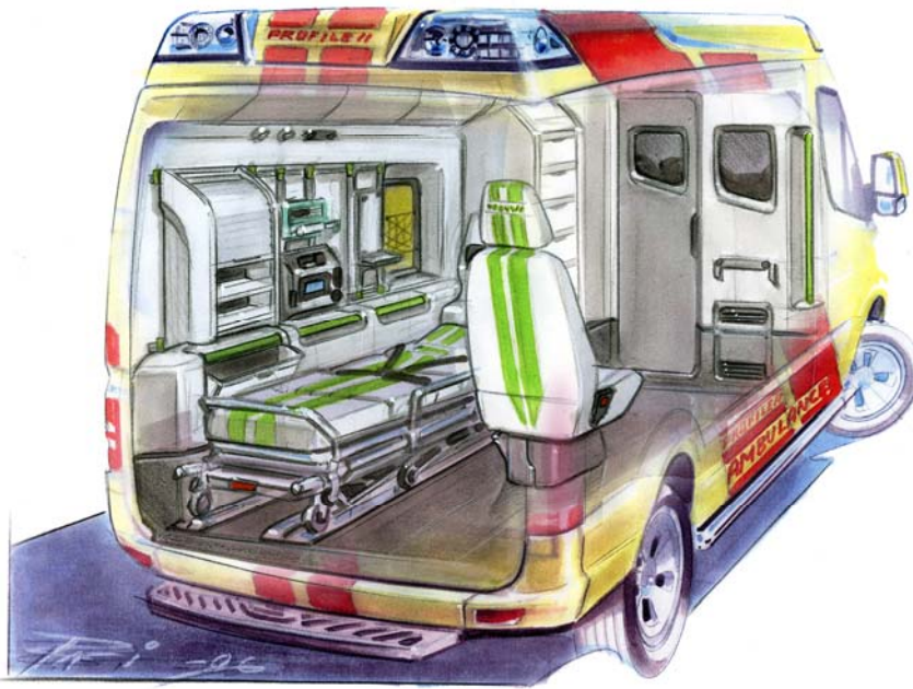
FIGURE 120. The basis of an ambulance is an unfurnished van whose roof is cut open and a new roof element is installed. When looking into the treatment area of an ambulance, everything there belongs to the delivery entity of the ambulance factory. The figure illustrates the Profile Genios ambulance.
