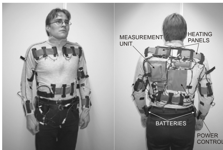
Figure 19. First heating prototype.
