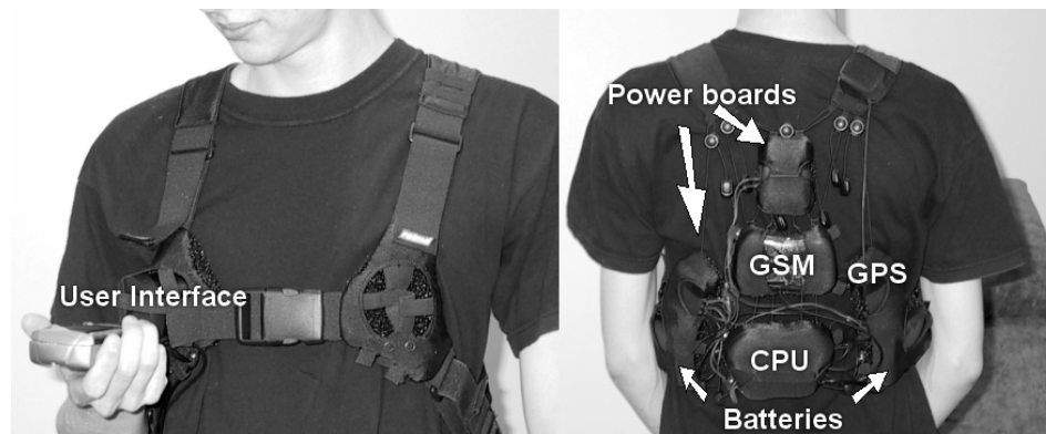
Figure 14. Supporting structure and main electronics components [P2].
