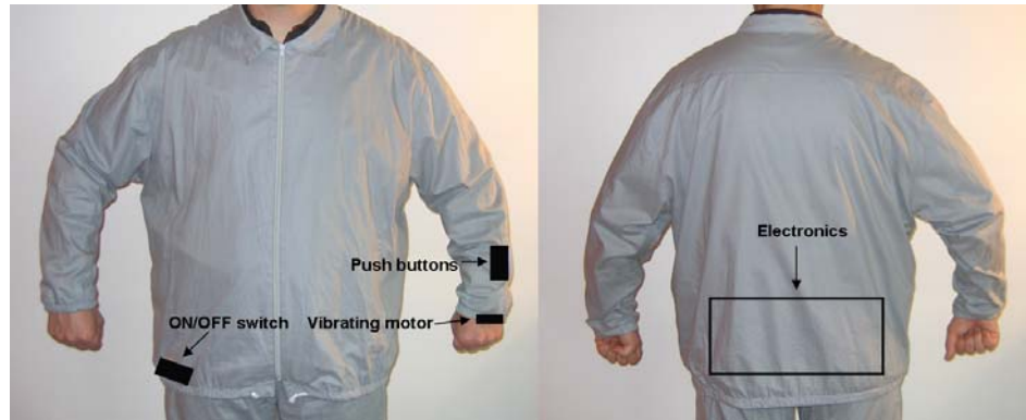
Figure 24. Bioimpedance measurement system [P6].
