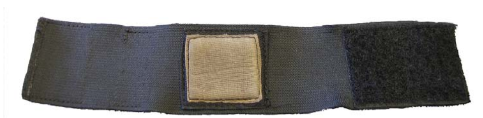
Figure 25. Textile electrode utilized in bioimpedance measurements [P6].
