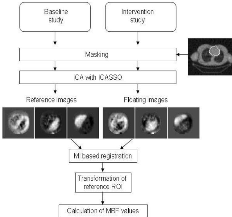
Figure 5.1: Schematic representation of the developed approach to align two dynamic studies.
