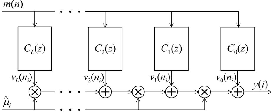
**Fig. 2.6** The Farrow structure for polynomial-based interpolation filter.
