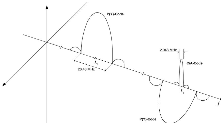
**Fig. 3.3** GPS signal spectrum (positive side).
