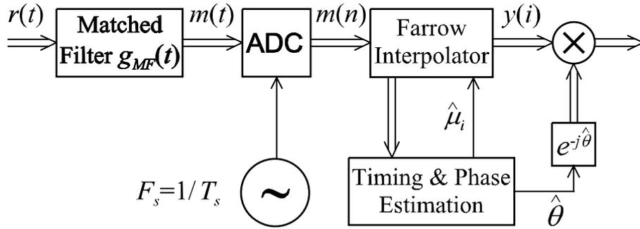
**Fig. 2.4** Digital receiver with non-synchronized sampling.
