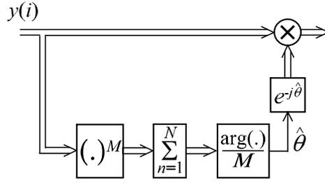
**Fig. 2.10** NDA carrier phase estimation scheme for M-PSK modulations.
