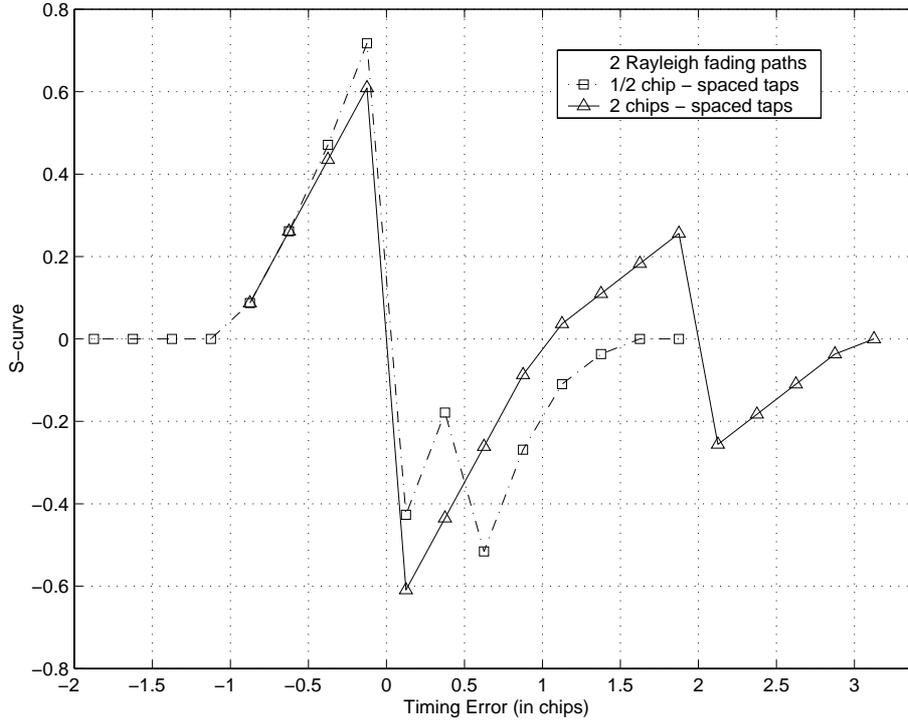
**Fig. 3.5** Non-coherent DLL S-curve for a multipath channel.
