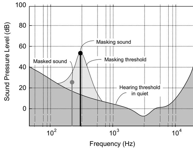
Figure 5. Masking effect illustrated in frequency domain.
