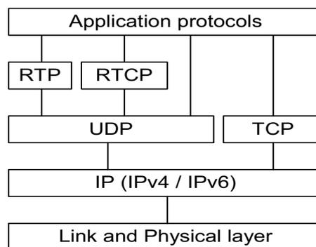
Figure 2. Typical protocol configuration for real-time transport over IP networks.
