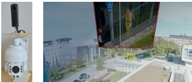
Figure 1: Left: a stationary 360° camera and a superzoom PTZ surveillance IP camera on a tripod.
