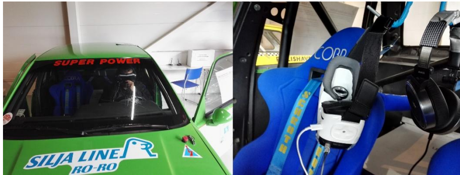
Fig. 4. In the 360° rally simulator installation, the user is able to sit in a real car and experience a rally stage through VR glasses and headphones.
