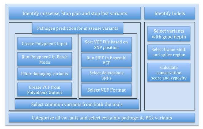
Figure 12. Pathogen Prediction pipeline for Indels and SNPs.
