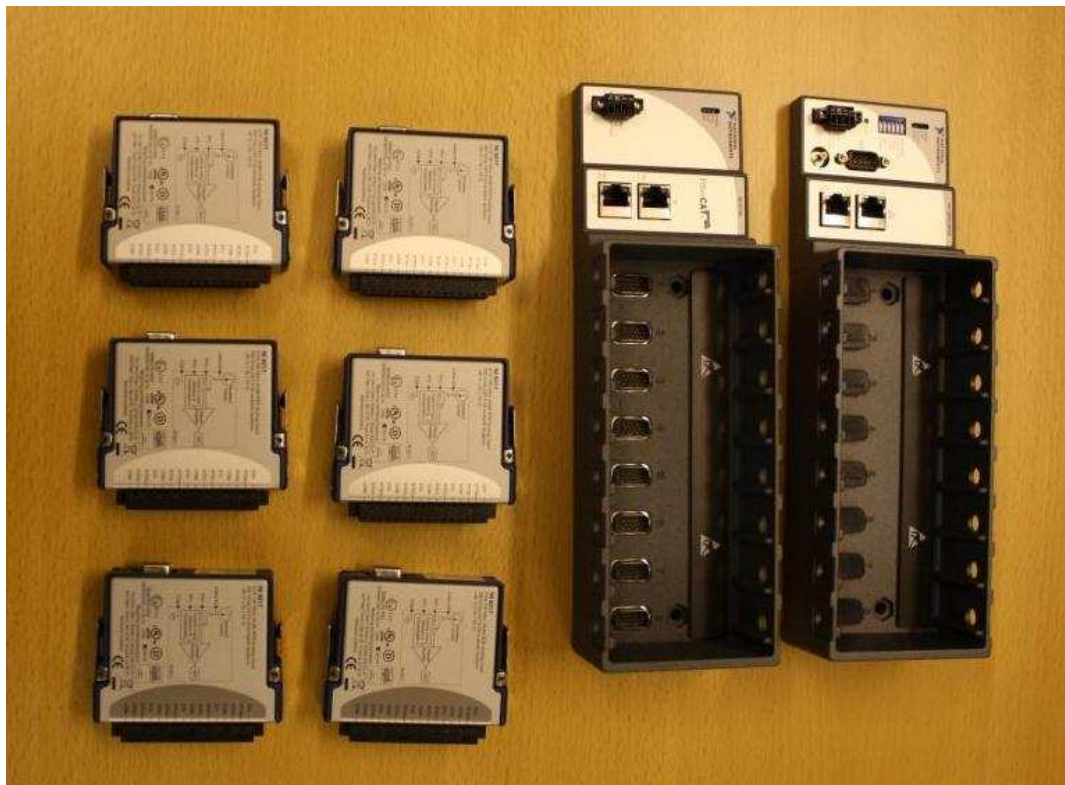
Figure 5.12. Components of the data-acquisition system during the mounting process.
