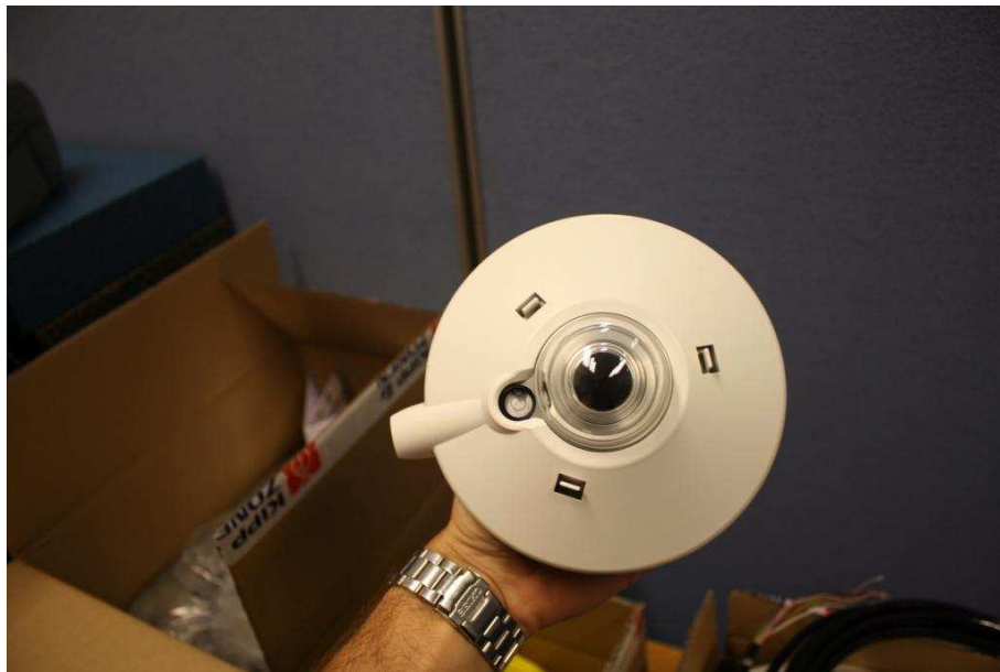
Figure 5.6. Kipp&Zonen's pyranometer CMP22 mounted under the cover of the CV3 ventilation unit.
