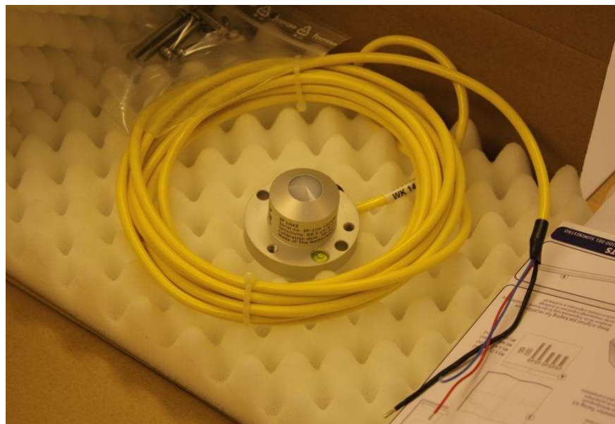
Figure 5.9. Photodiode-based pyranometer SP Lite 2 during the mounting process in the laboratory.
