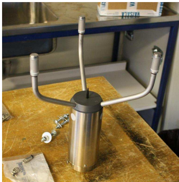
Figure 5.5. WS425 ultrasonic wind sensor during the mounting process.
