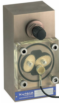
Figure 2.20: SR oval gear meter. Taken from [Kytölä 10].
