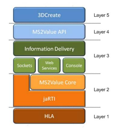
Figure 16 Architecture for the HLA-DS tool.
