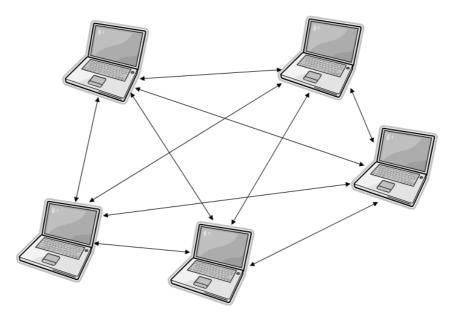
*Figure 10* In a Peer-to-Peer architecture each computer is connected to several computers without a centralized server.
