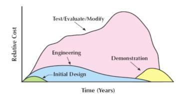
*Figure 1* Iterative Prototyping consumes billion of dollars and years of development for complex products. M&S can drastically reduce those costs [IMTI 2000].
