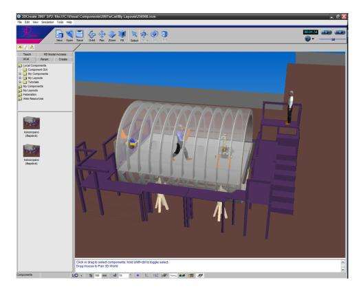
*Figure 7* Ergonomic analysis is possible by the inclusion of human models to the simulation environment.
