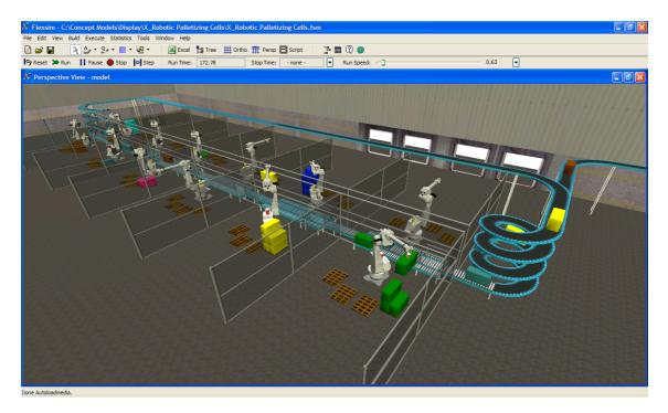
Figure 5 Flow of products can be analyzed and optimized by using simulation.
