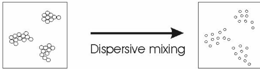
Figure 2.3.4.2–1 Dispersion of fillers in matrix [59].
