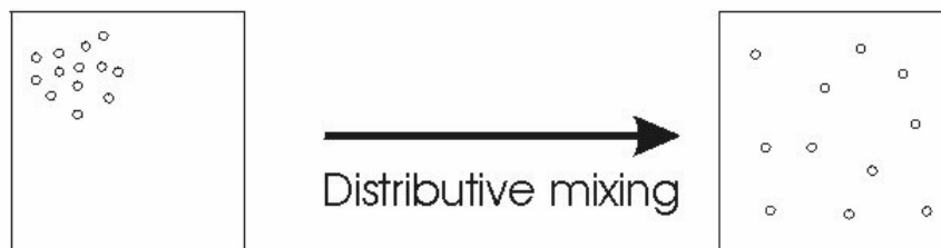
Figure 2.3.4.3–1 Distribution of fillers in a matrix [59].
