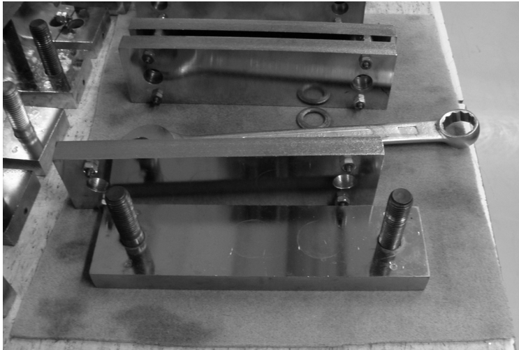
Figure 3.3.4–1 Compression set testing equipment.
