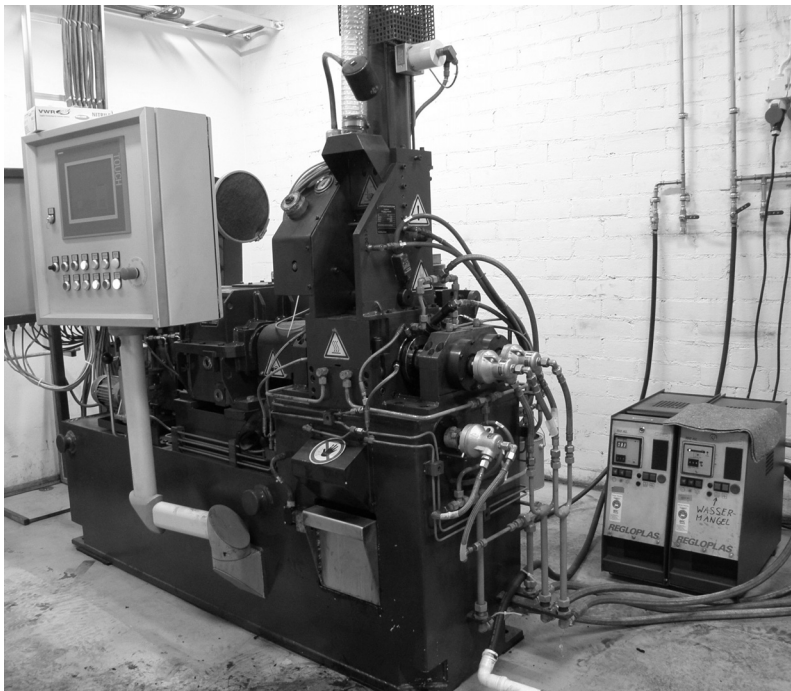
Figure 3.2.1–1 Internal mixer used for the compounding of the nanocomposites.
