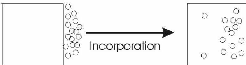
Figure 2.3.4.1–1 Incorporation of fillers in a matrix [59].
