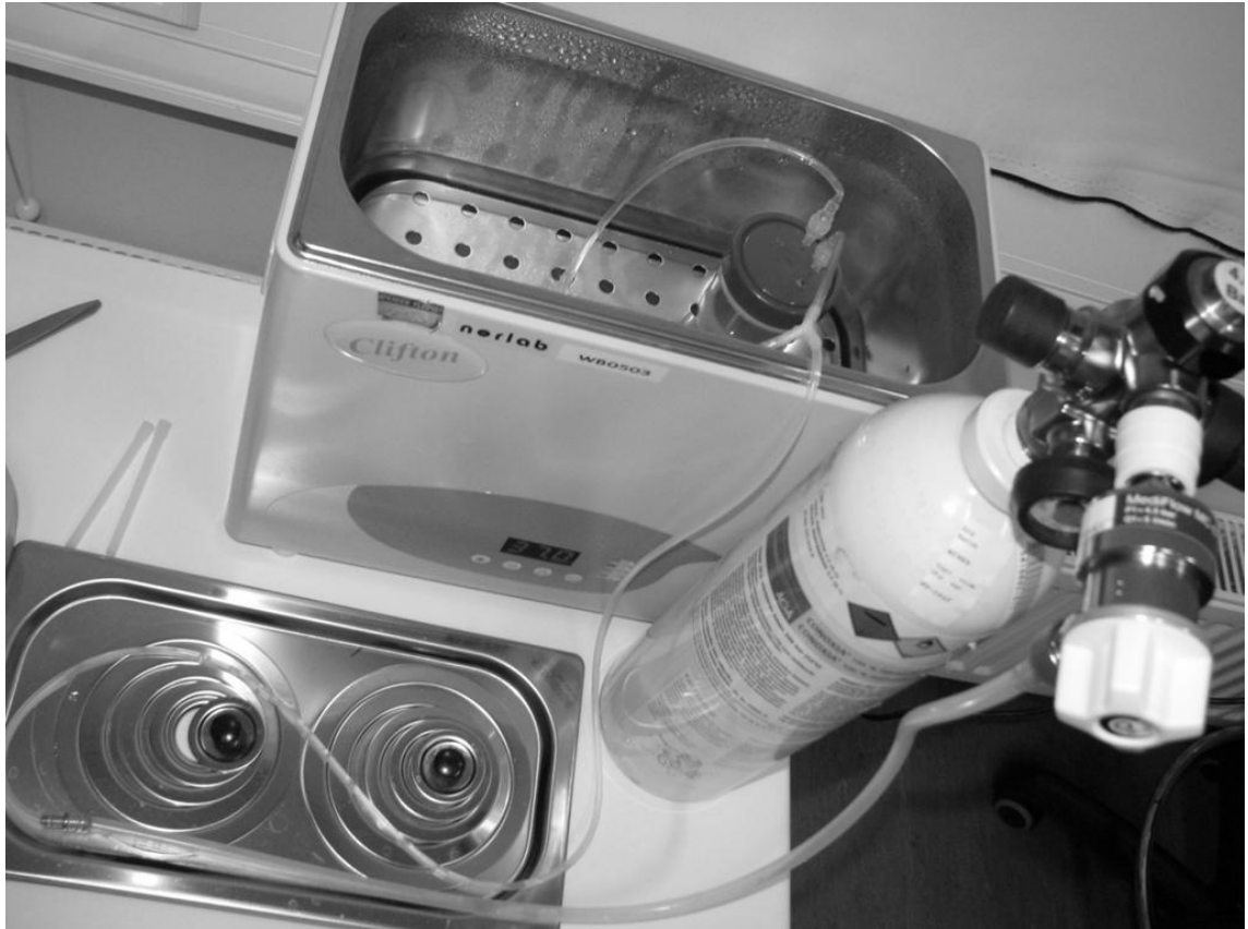
Figure 3.4. Heating Ames medium to 37 °C and oxygenating it. The lid of the water bath is removed for photographing purposes.
