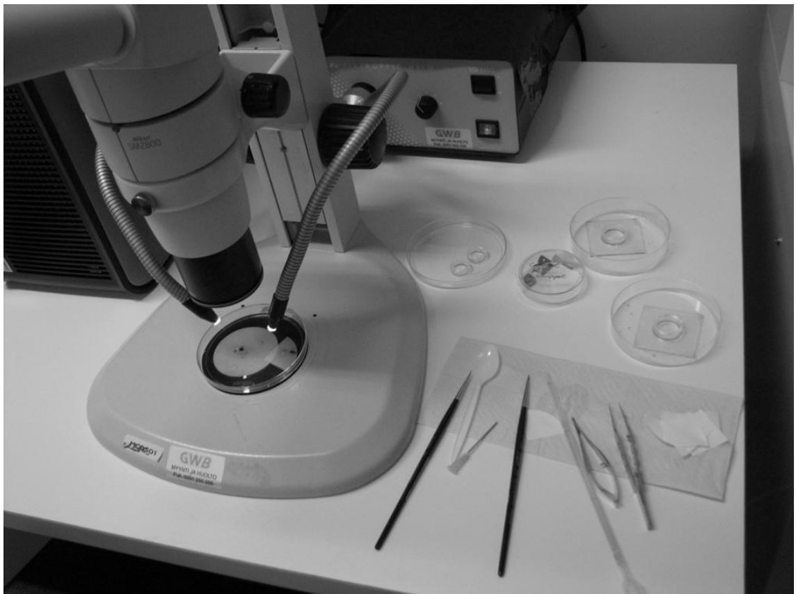
Figure 3.7. Preparation site. Preparation tools are placed on the right side of the dissecting microscope. MEAs, carriers and PDMS rings are on Petri dishes behind the tools.
