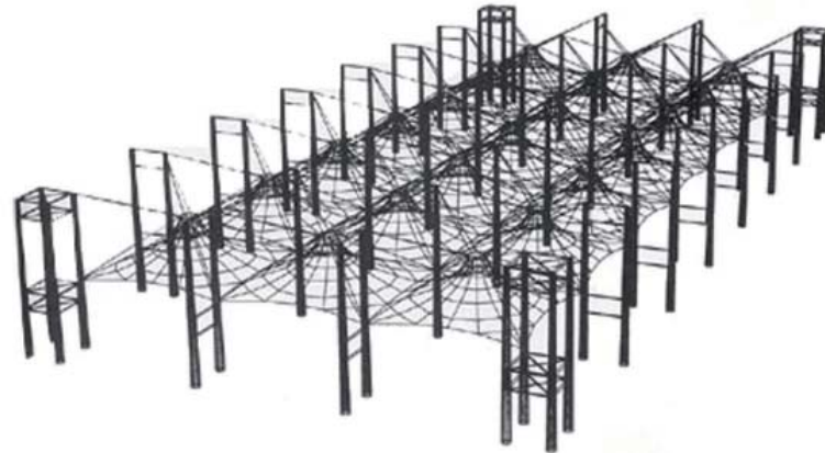
30b The structural system simplified. (Berger 2004, 98)
