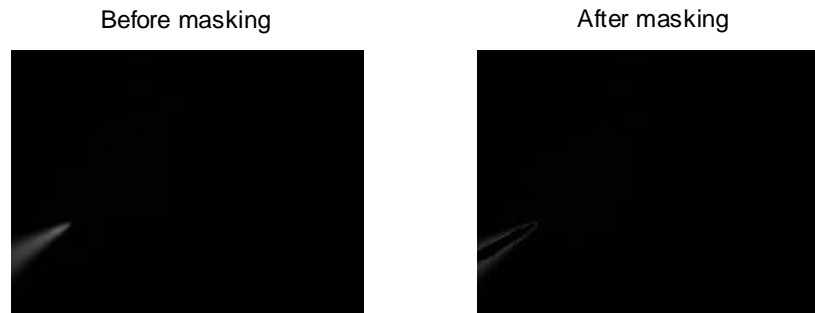
Figure 5.5: Masking the pipette out. The original image shown in the left and the masked image shown in the right. For illustration purposes, a good mask is not applied and the borders of the pipette are clearly visible.
