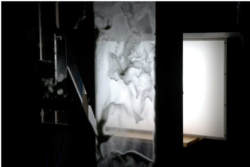
Figure 6.11. Continuous lighting setup. The CFB riser and loop seal lit by a pack of high frequency fluorescent tubes.
