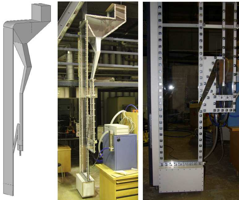
Figure 3.1. A schematic and pictures of the 2D pilot scale CFB and the lower portion with the windbox and the loop seal. Picture Matias Guldén (2008).
