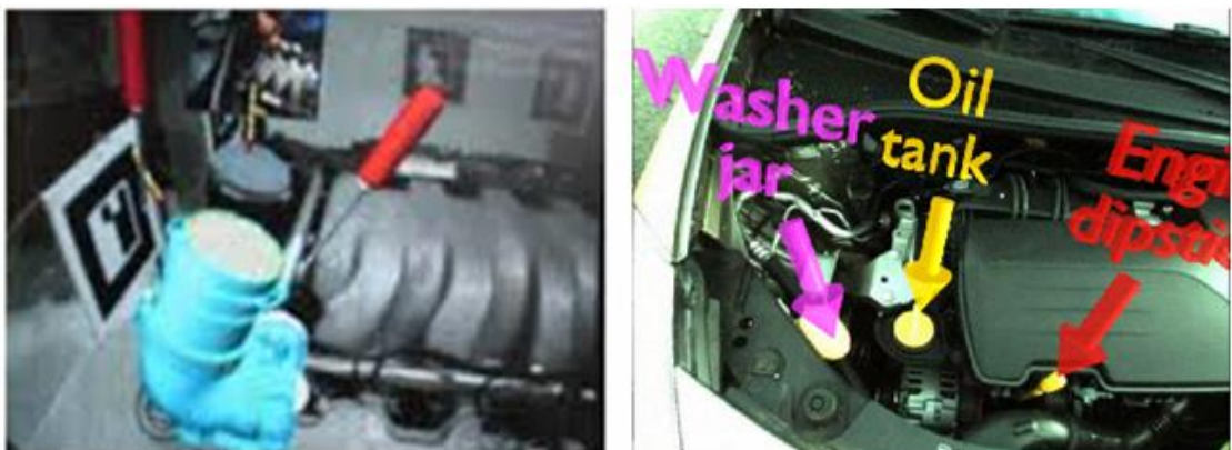
Figure 6. Maintenance assistance through a) marker based AR [11] and b) markerless AR [12]
