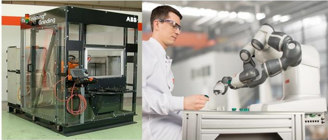
Figure 9. a) industrial ABB robot in a cell [24], b) ABB cobot interacting with an operator [24]
