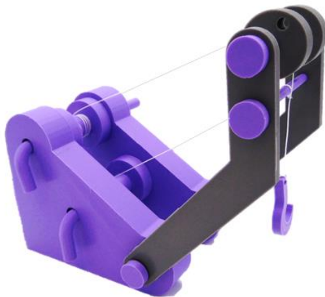
Figure 31. 3D printed prototype of the crane
