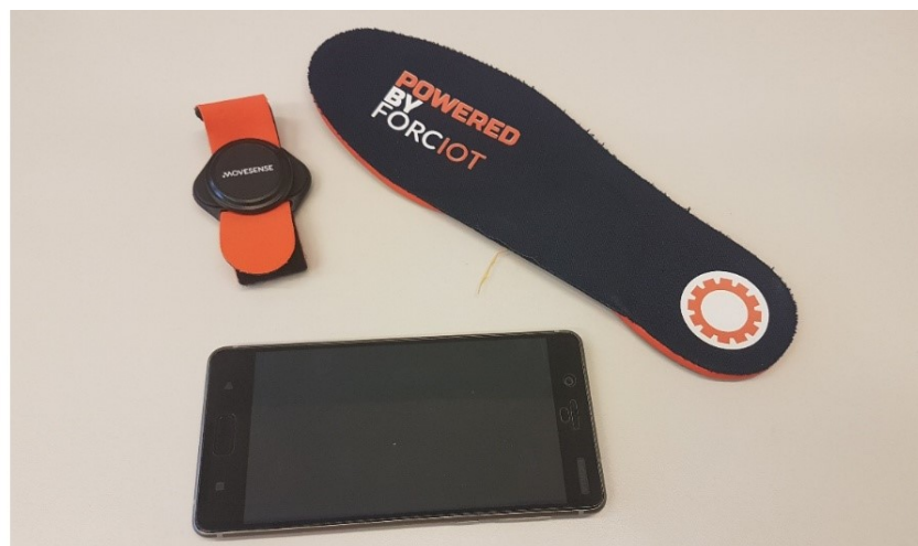
Figure 1. Devices used: Suunto Movesense sensor (top left), Forciot Smart insole (top right) and cell phone (bottom) [8]
