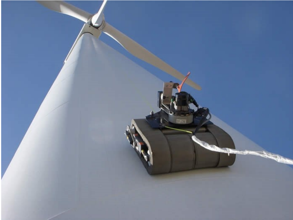
Figure 2. IMC's The Climber robot inspecting wind turbine pole [17]
