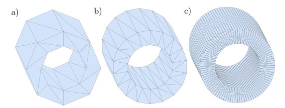
**Figure 2.5** A circular tube triangle mesh model with different level-of-detail: a) 64 triangles b) 144 triangles c) 768 triangles.
