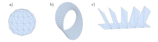
**Figure 2.4** Visualization of a) manifold mesh, a closed sphere, b) Möbius strip, manifold mesh with boundary, c) non-manifold mesh.
