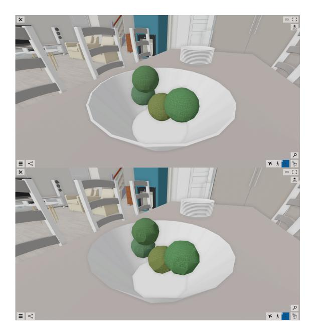
Figure B.2 Original and simplified Vertex CAD building model. Round objects are simplified to a significant extent.
