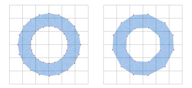
**Figure** 3.1 Visualization of vertex clustering, where clusters (left) are merged to a single vertex, which is positioned to the average position of cluster vertices (right).
