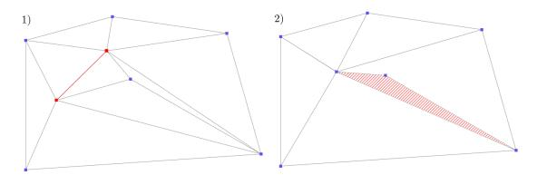
Figure 4.3 Visualization of 1) invalid edge collapse operation, 2) where the triangle in red stripes is non-manifold after the collapse of the red edge.
