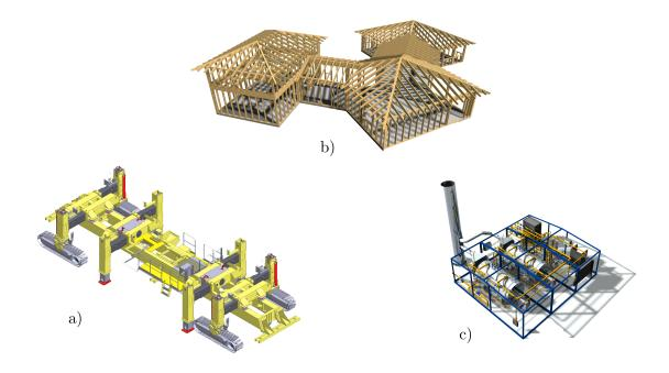
**Figure 1.1** Models designed using Vertex CAD software: a) mechanical assembly b) building framing c) plant design. [1]
