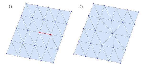
**Figure 3.3** Visualization of edge decimation. The edge in red is 1) selected and 2) collapsed.
