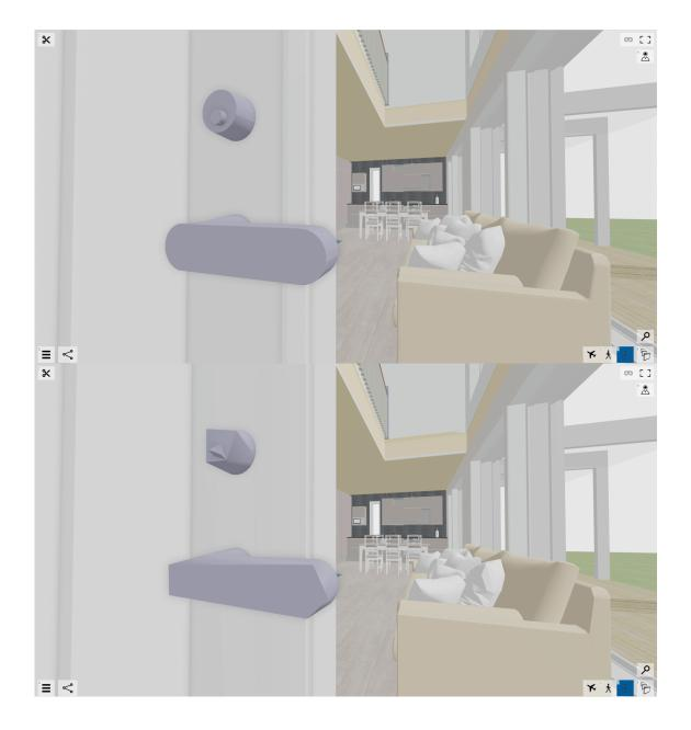
**Figure B.3** Original and simplified Vertex CAD building model. Door handle which contains lots of high frequency detail is simplified, while all low frequency detail such as walls, doors and other decorative objects are in place.
