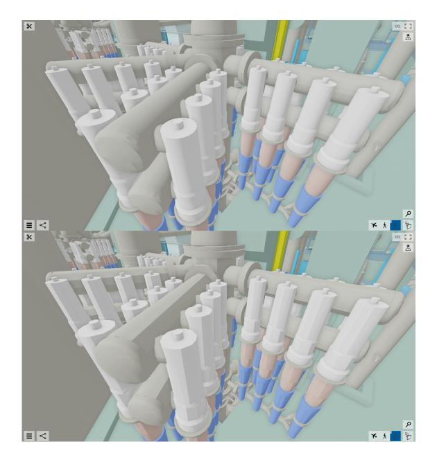
**Figure B.4** Original and simplified Vertex CAD plant model. Again, round elements benefit from the simplification, the overall shape is still remained while great amount of geometry has been decimated.
