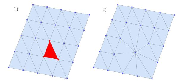
**Figure 3.4** Visualization of triangle decimation. The triangle in red is 1) selected and 2) collapsed.
