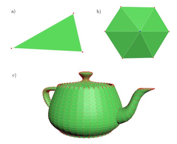
Figure 2.3 Visualization of a) triangle, b) surface and c) mesh model.
