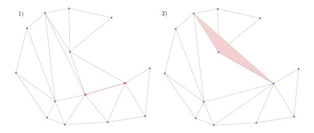
Figure 4.2 Visualization of 1) invalid edge collapse operation, 2) where the triangle in red stripes is flipped after the collapse of the red edge.
