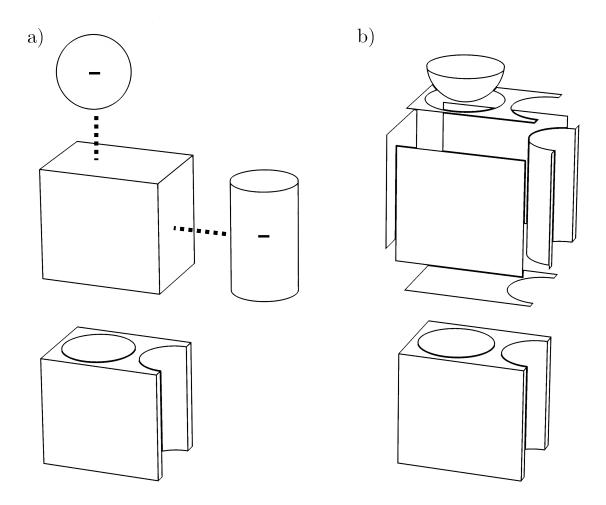
Figure 2.2 Two methods of solid modeling: a) CSG and b) B-rep.
