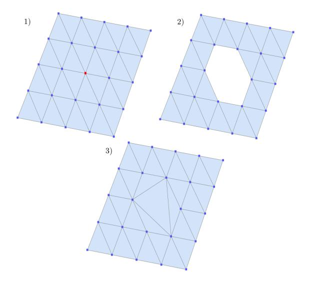
**Figure 3.2** Visualization of vertex decimation. The vertex in red is 1) selected and 2) removed. Finally, 3) the resulting hole is patched.
