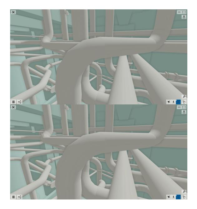
**Figure B.5** Original and simplified Vertex CAD plant model. In this specific plant model, piping mesh is from non-manifold surfaces and due to constraints, cannot be simplified.
