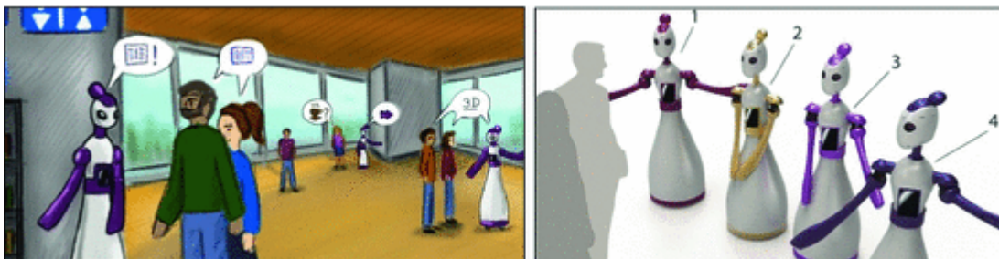
Figure 2.3. (a) Conceptual art of IOMI interacting with groups of people and (b) set of gestures: (1) Greeting Stance; (2) Waiting Stance; (3) Follow-me Stance; (4) Pointing Stance. Adapted from “Introducing IOMi - A Female Robot Hostess for Guidance in a University Environment”, by E.Onchi, 2016, 8th International Conference, p. 765. Copyright [2016] by Springer International Publishing.
