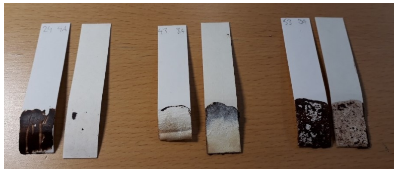
Figure 2. Examples of modes of failure. From left to right: adhesive failure, cohesive failure in adherend, cohesive failure in adhesive.
