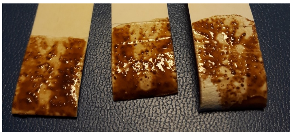
Figure 32. Co1-CPT HMA on cardboard after opening. Co1-CPT did not achieve homogeneity, and small tannin particles can be seen.
