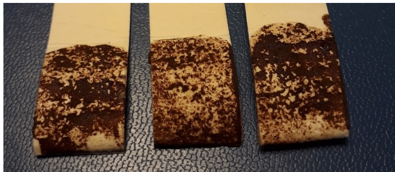
Figure 31. Co1-CST HMA on cardboard after opening. Co1-CST created a seemingly homogenous dark brown paste.
