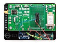
(a) Final receiver structure with EVB in RSSI mode.
