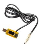
(a) ZY1273 USB power meter with TTL to USB cable
