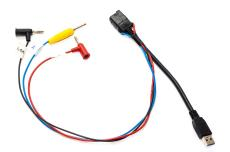
(b) USB cable with parallel connection for multimeter measurments
