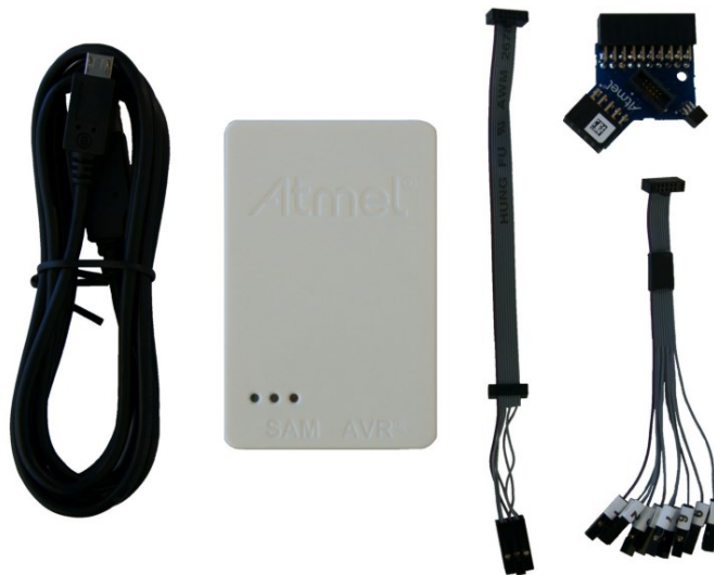
Figure 6. Atmel ICE JTAG programmer and adapter cables [8, p. 7] were used for programming the target MCU and doing in-system debugging.
