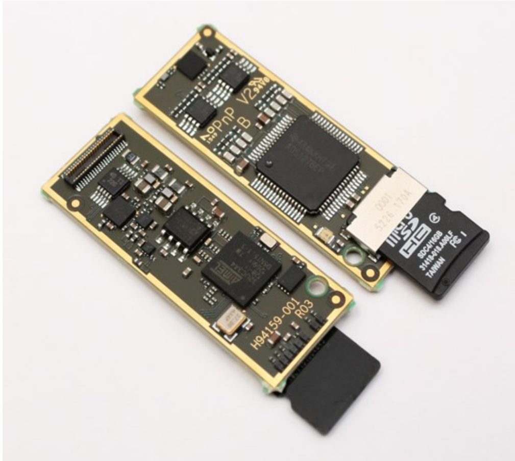
Figure 4. Photo of the final revision PnP DAQ card hardware shows both sides of PCB fully assembled with components. The PCB has 8-layer any-layer micro via high-density stack-up to meet demanding size requirements.
