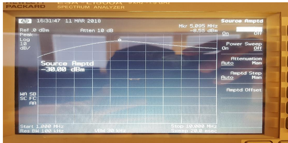
Figure 39: Spectrum Analyzer result for -30dBm Source Amplitude, Gain = ~22dB, at 5MHz Frequency
