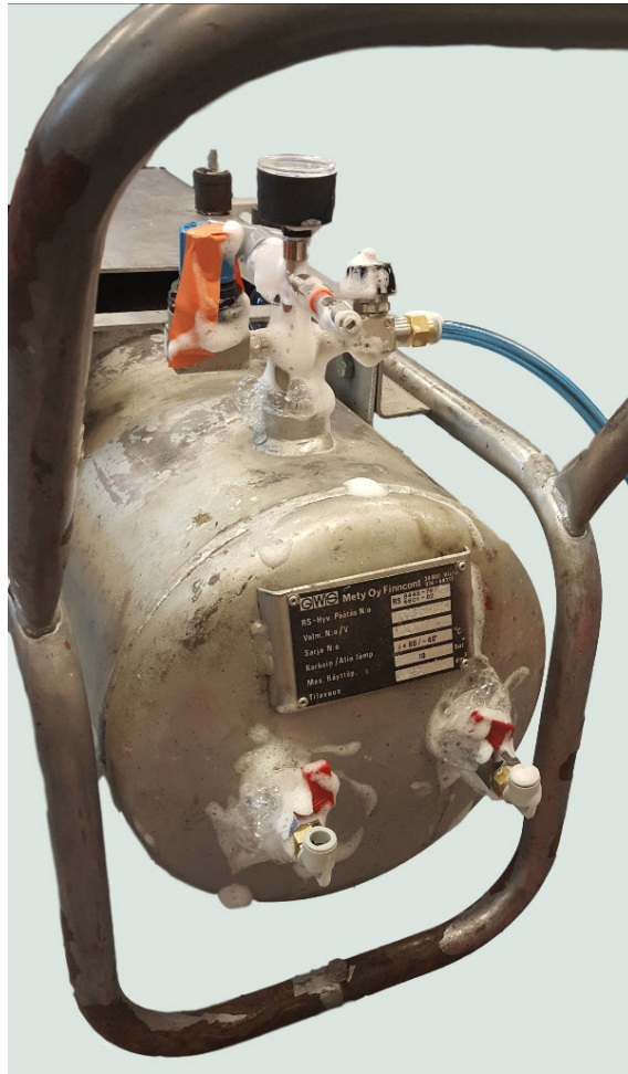
Figure 3.8 Tank while being tested for possible leakges
