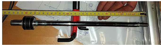
(a) Piston CoM measurement
