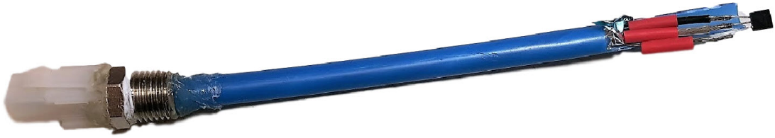
Figure 3.18 LM35 temperature sensor for the reservoir
