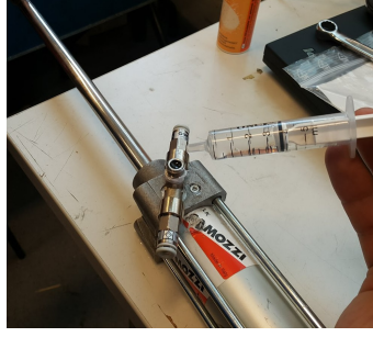
Figure 6.25 Measuring dead volume of chamber B of a cylinder
