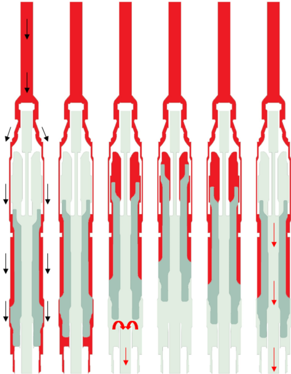
Figure 7. Piston cycle excluding flushing. High-pressure air is marked with red, atmospheric air with light green and piston with dark green. Black arrows indicate the initial flow direction and red arrows the discharge of high-pressure air.
