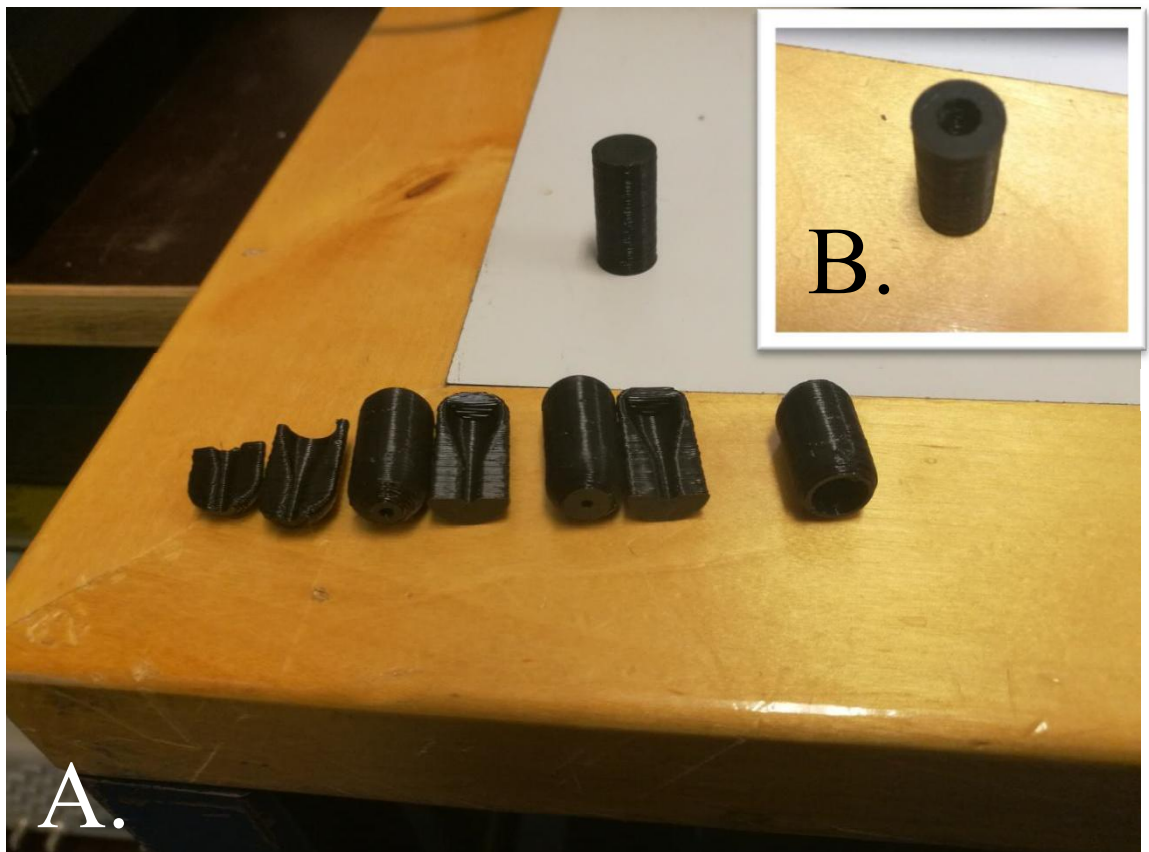
Figure 27. A. First set of printings. Capsules printed into half show the wine bottle shape inside the capsules. B. The first prototype capsule cylinder with an open head.
