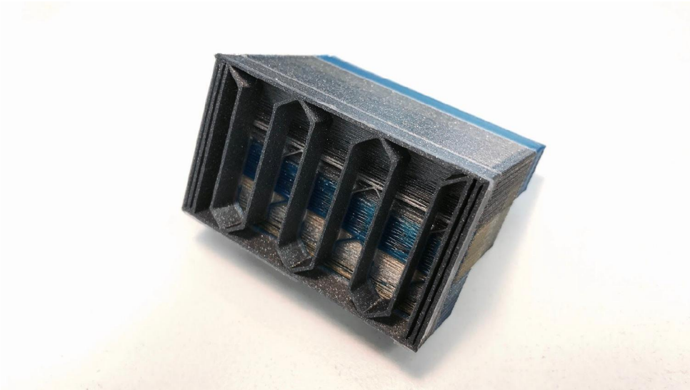
When filament change is not needed, smart wipe tower is hollow.
