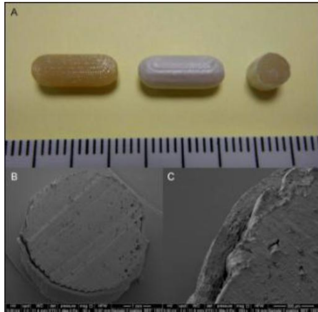
Figure 13. A. Printed PVA caplet, coated printed PVA caplet and a cross-section of a coated caplet. B.,C. SEM images of the coated caplet cross-section surface. Image source: [23].
