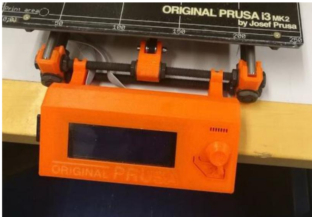
Figure 24. Printer user interface, power off. Note the control knob on the right side of the LCD panel.
