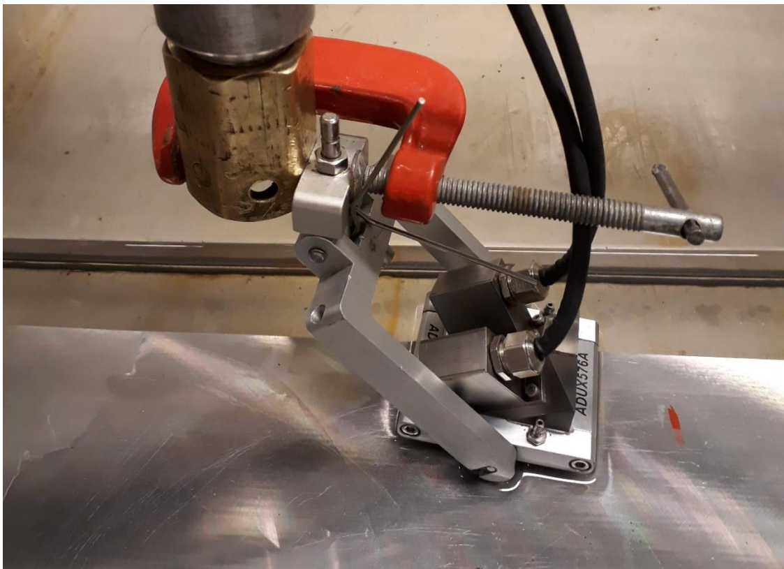
Figure 32. Scanning setup for the ultrasonic inspection
