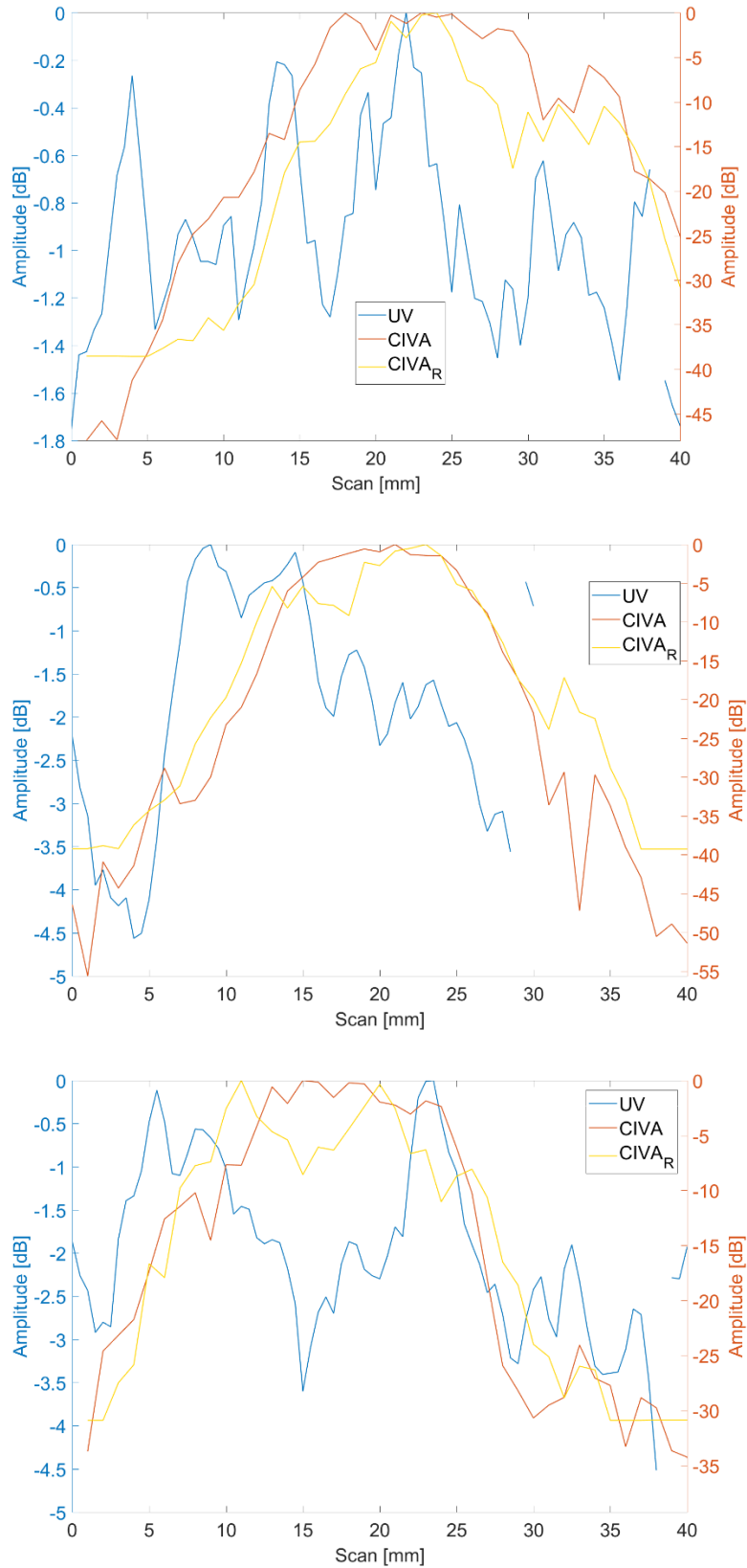
Figure 62. Results for flaw 1 with different amplitude axes, top for +10^\circ , middle for 0^\circ and bottom for -10^\circ probe tilt angle.
