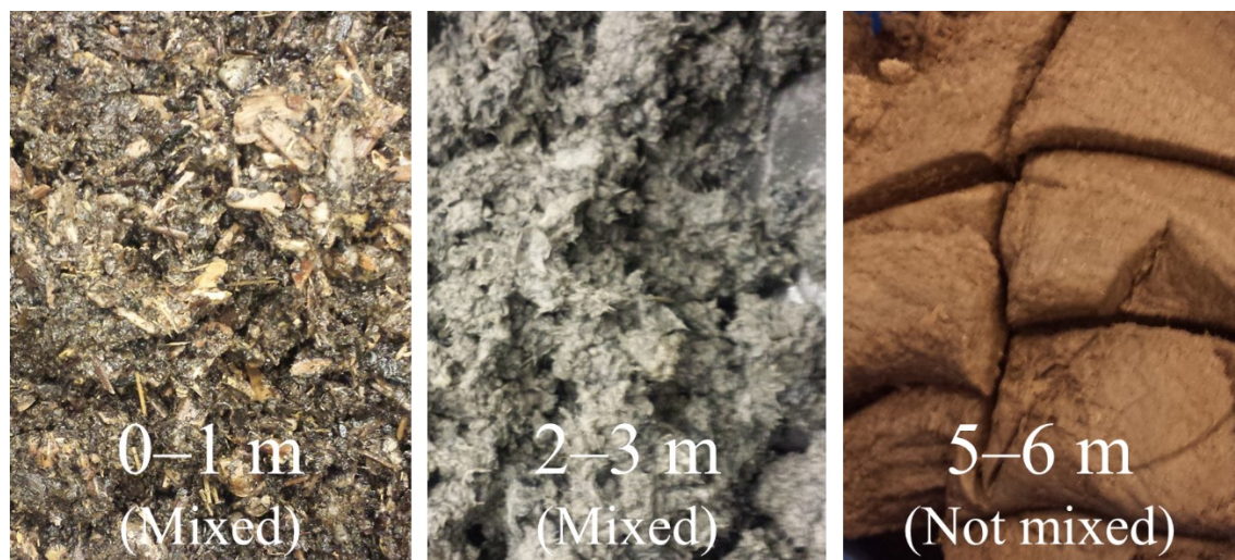
Figure 8. The visual appearance of the sedimented fibers. The layers closest to surface are rich in wood pieces and solids (on the left), whereas deeper the sediment has higher moisture content and the fibers are softer (in the center and on the right), forming a felt-like structure (on the right).
