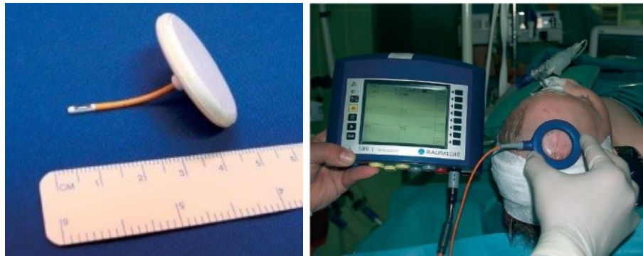
Figure 5: A) Raumedic's wireless ICP sensor. B) Wireless reading of the ICP. [24]
