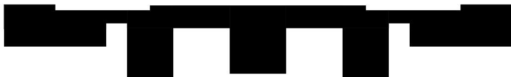
Figure 22. The layout of the low pass filter
