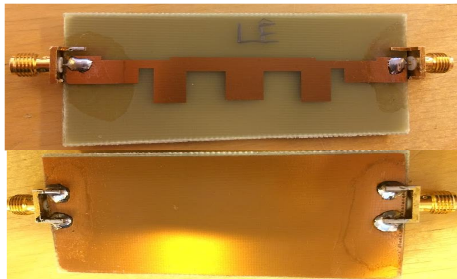
Figure 8. The low pass stub filter
