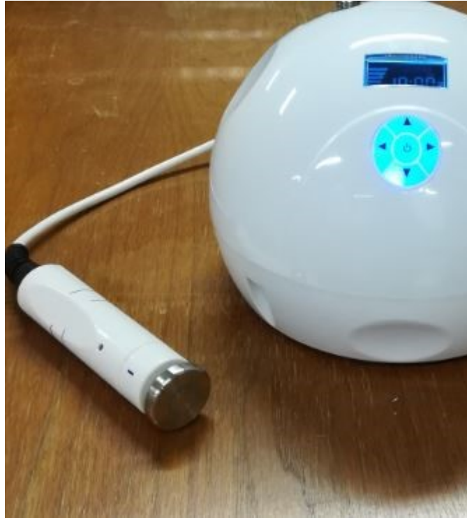
Figure 4. RF beauty care appliance Panda Box and its larger electrode, diameter of 3,4 cm.
