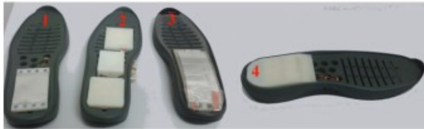
Figure 21. Four shoe energy harvester configurations. (Gatto and Frontoni 2014)
