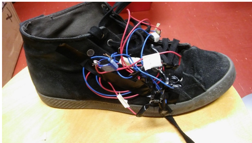
Figure 61. Supercapacitor connected to the piezoelectric elements that are inserted in the shoe.
