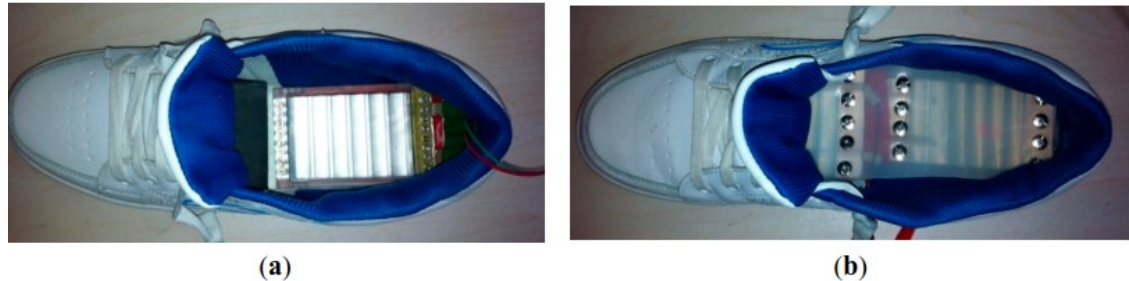
Figure 25. Energy harvester a) prototype 1, b) prototype 2. (Zhao and You 2014)
