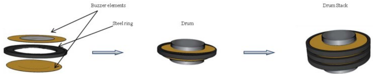
Figure 27. Schematics of the drum transducer. (Mishra et al. 2017)
