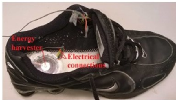
Figure 33. Stacked diaphragms with the pre-stress mechanism placed in a shoe. (Leinonen et al. 2016)
