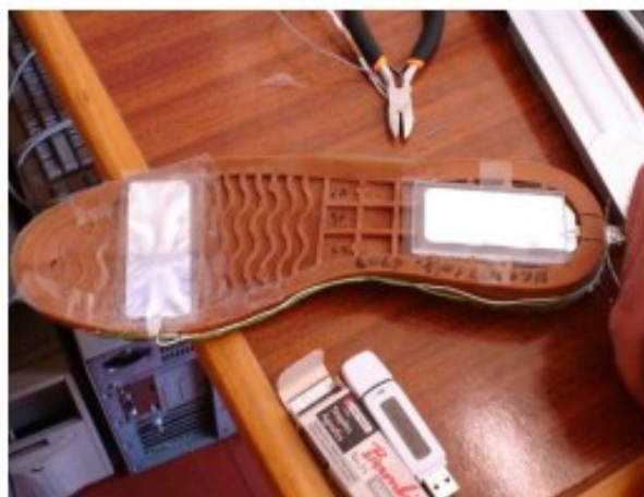
Figure 20. PVDF films attached to the shoe. (Rocha et al. 2010)
