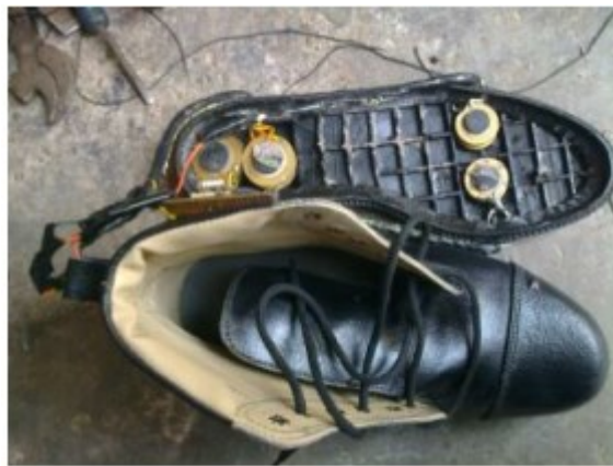
Figure 28. Drum transducers mounted in a shoe. (Mishra et al. 2017)
