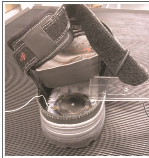
Figure 30. The cymbal energy harvester inserted in a shoe. (Palosaari et al. 2012)
