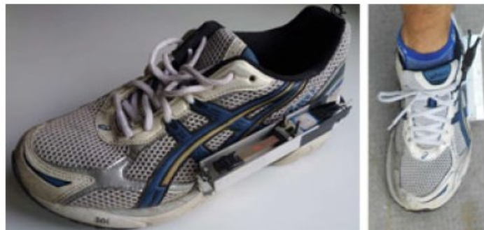
Figure 16. Cantilever type energy harvester attached to a shoe. (Camilloni et al. 2016)
