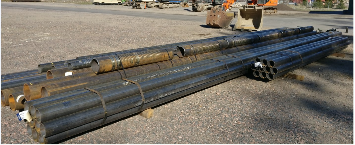
Figure 25. RDs pile elements
