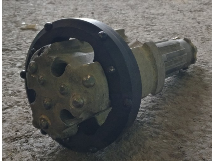
Figure 29. The pilot bit and the reamer from Atlas Copco
