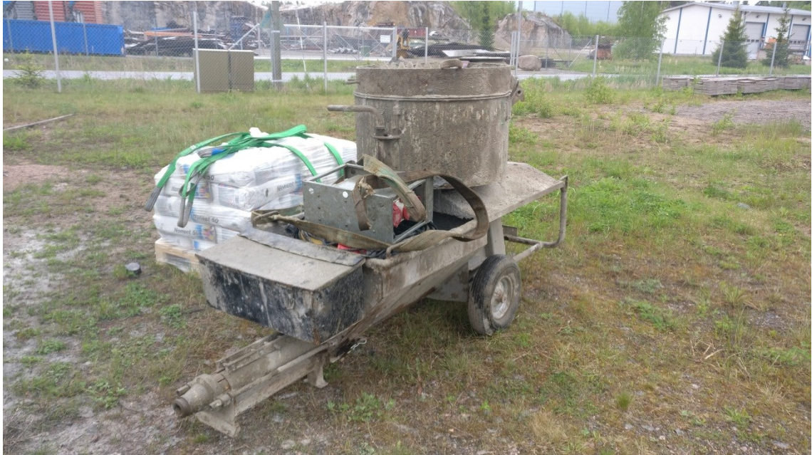
Figure 37. The grout mixer
