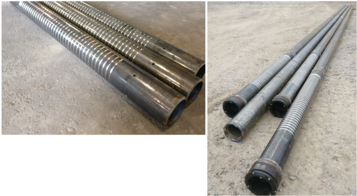
Figure 27. Grooved part of the test pile and final RDs 140/10 piles
