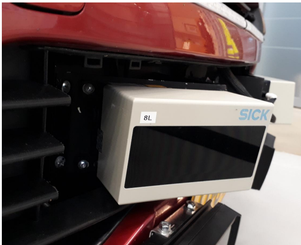
Figure 2. Sick LD-MRS LiDAR mounted on Marilyn's front bumper.
