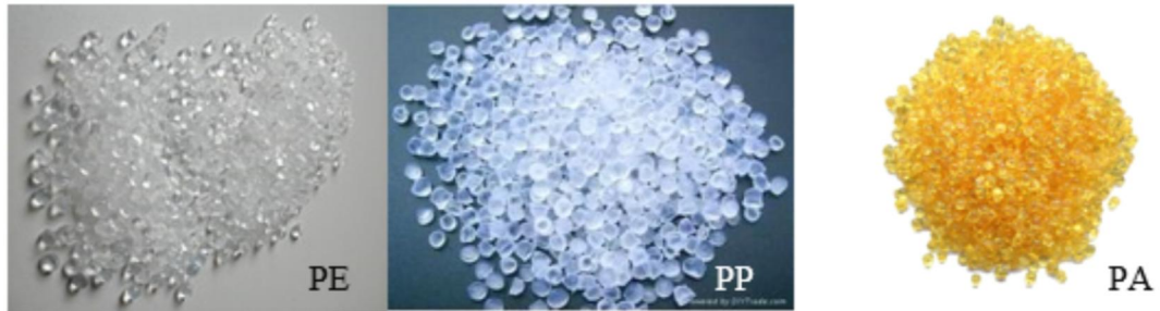
Figure 7. Most common thermoplastic matrix materials. [7] [8] [9]
