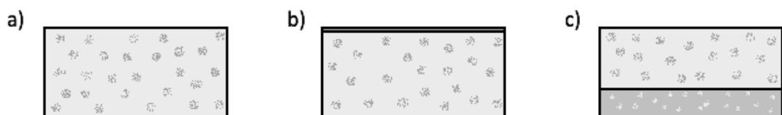
Figure 2. Schematic picture of the cross-sections of different flooring types: a) homogeneous structure, b) layer structure, i.e. homogeneous layer with thin wearing course of PVC or PUR and c) heterogeneous structure.
