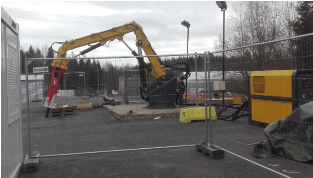
Figure 4.1 The pedestal rock breaker boom studied in this thesis.
