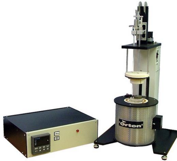
Figure 15. The parallel-plate viscometer for viscosity measurement [Or, 07].
