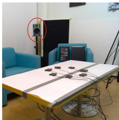
(a) Photograph of the recording case setup. The used loudspeaker is circled.
