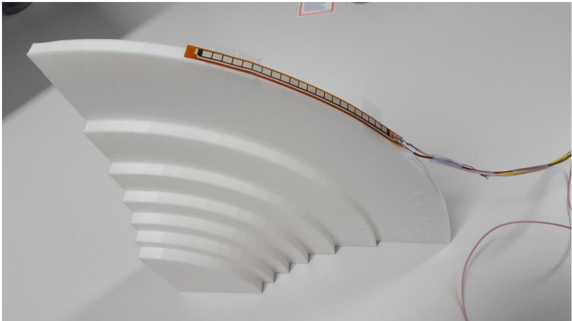
Figure 10: 3D printed setup for calibration
