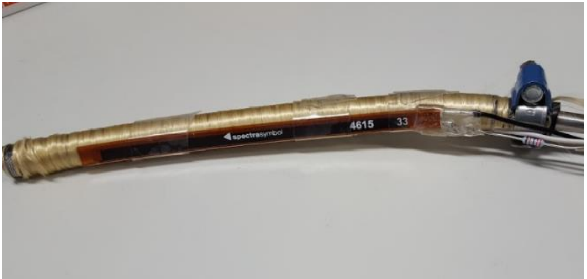
Figure 13: Failed method to attach sensor as wounding the tape caused difficulty in appropriate sensor bending
