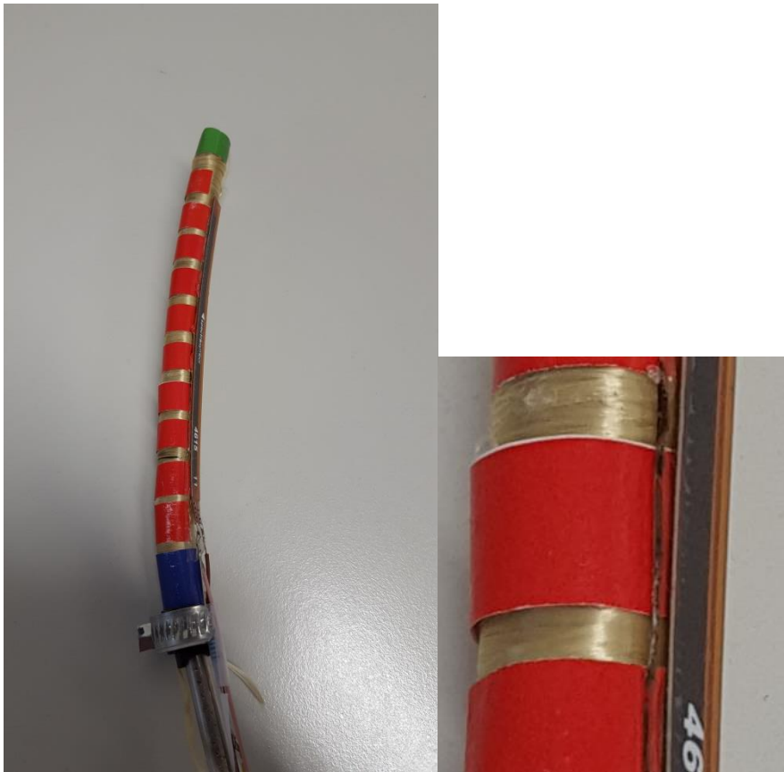
Figure 14: Correct attachment method for sensor
