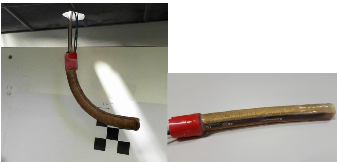
Figure 12: Describing the low bending due to embedding sensor completely inside the robot and coating it with rubber
