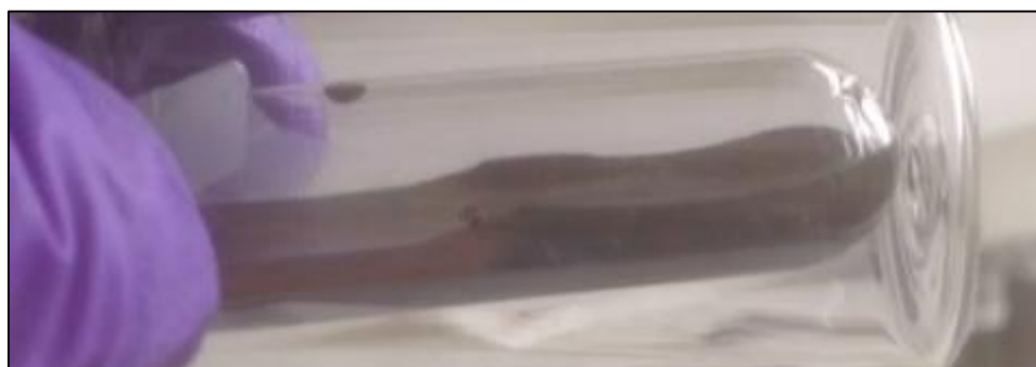
Figure 17. Purified graphene after 8 weeks without any sedimentation and agglomerate
