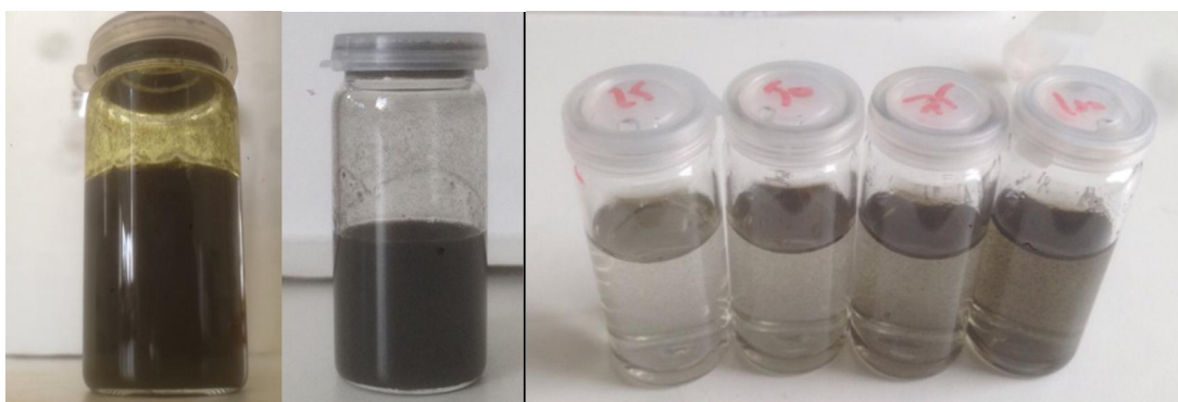
Figure 9. Unpurified and purified graphene dispersion along with the diluted versions. (From left to right: Unpurified aqueous graphene dispersion stabilized by stabilizer 3, stabilizer 1, and Dilutions-stabilizer 1).
