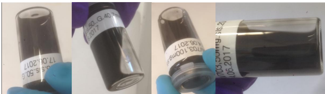
Figure 10. Pictures of stabilizer 1-stabilized graphene without any visible agglomeration or sedimentation.
