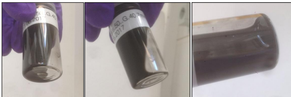
Figure 14. The sedimentation behavior of stabilizer 1-stabilized graphene by time (from left-right: after 48 hours, two weeks and a month)
