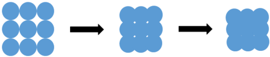
Figure 4. Illustration of sintering process. Based on (Ertuğ 2013, p. 93).
